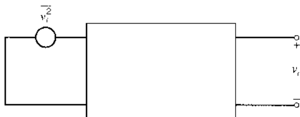
Figure 11.41 Circuit with equivalent input noise voltage generator.
