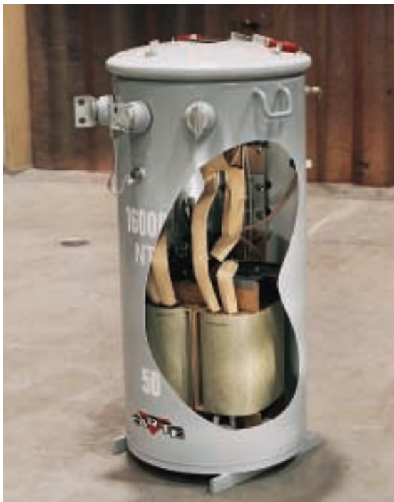
FIGURE 24-3 Distribution transformer (cutaway view) of the type used by electric utilities to distribute power to residential and commercial users. The tank is filled with oil to improve insulation and to remove heat from the core and windings. (Courtesy Carte International Inc.)
