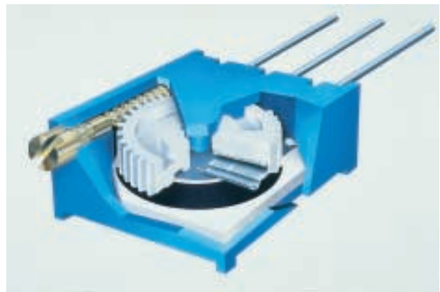
(b) Internal view of variable resistor.
