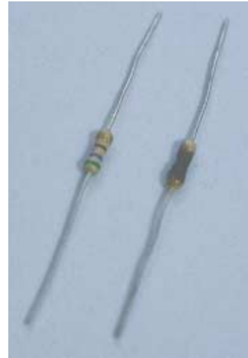
FIGURE 4–18 The resistor on the right has been damaged by overheating.
