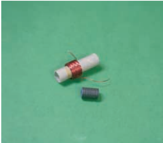
FIGURE 13–19 A variable inductor with its ferrite core removed for viewing.
