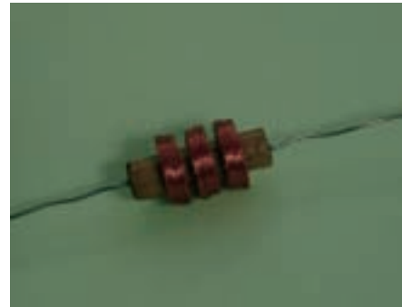
(b) Separating coil into sections helps reduce stray capacitance
