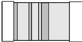
Figure 1.2 A surface mount resistor.
