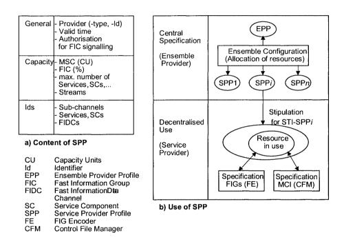
Figure 6.16 Management by means of service provider profiles
