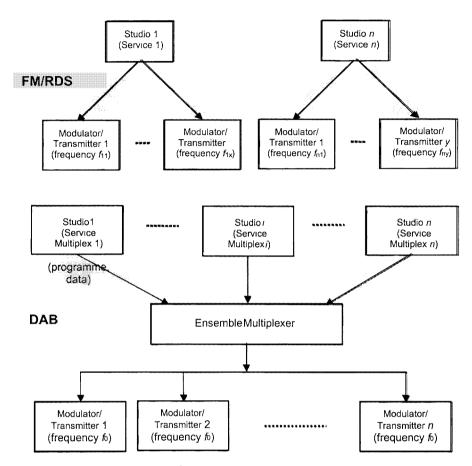
Figure 6.1 Network architecture of DAB versus FM/RDS
