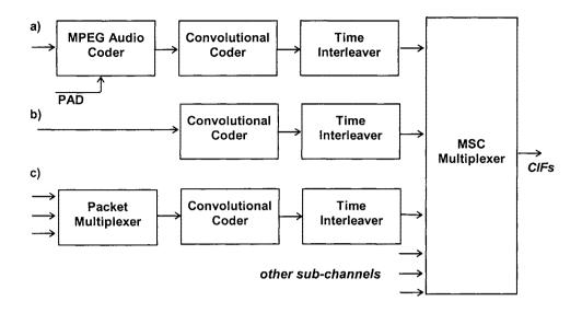
Figure 2.9 Generation of the common interleaved frames (CIFs) from a) an audio sub-channel, b) a general data stream mode sub-channel, c) a packet mode sub-channel.
