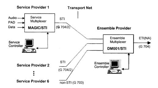
Figure 6.15 Structure of the collection network
