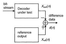
Figure 8.11 Audio conformance test procedure
