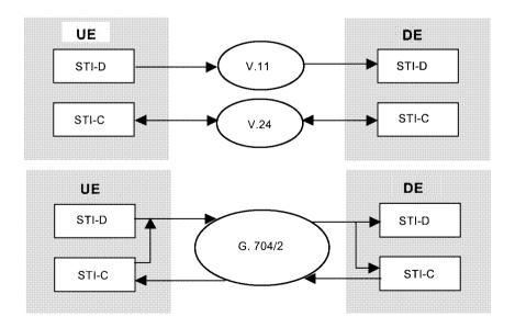
Figure 6.9 Physical connections of STI-D and STI-C (examples)
