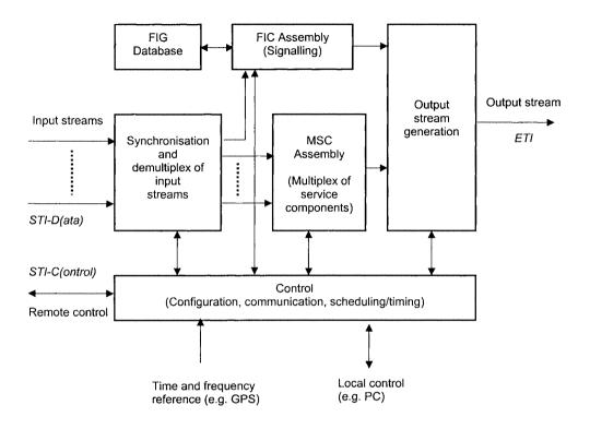
Figure 6.2 Conceptual block diagram of ensemble multiplexer
