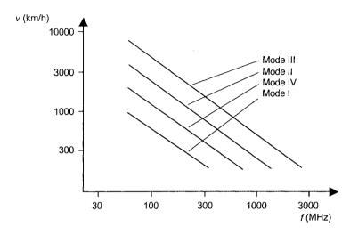
Figure 7.1 Interdependencies of maximum speed, frequency and DAB mode
