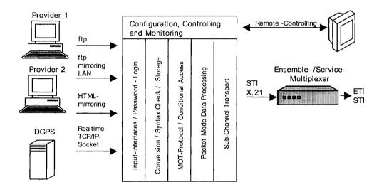
Figure 5.7 Packet mode inserter (based on the Multimedia Data Server developed by FhG)
