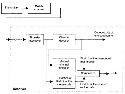
Figure 7.17 Generation of the pseudo-channel BER using a MSC sub-channel
