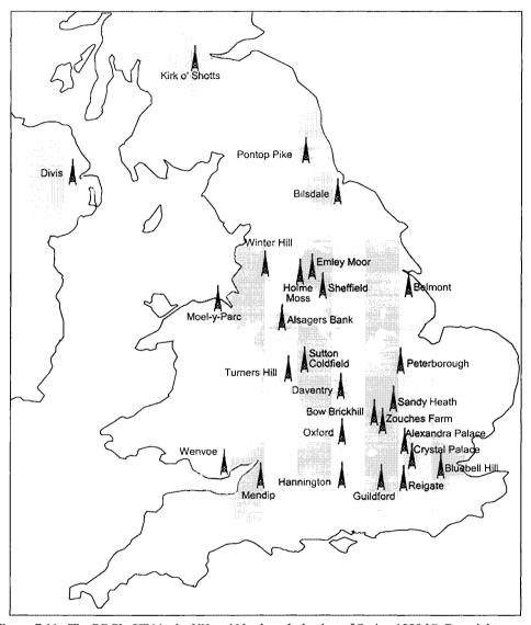
Figure 7.11 The BBC's SFN in the UK and Northern Ireland as of Spring 1998 [© Copyright British Broadcasting Corporation 2000. Reproduced by permission of the British Broadcasting Corporation]
