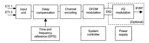
Figure 7.5 Block diagram of a COFDM modulator
