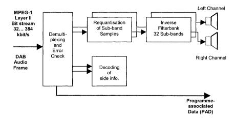
Figure 3.5 Block diagram of the MPEG-1 Audio Layer II decoder
