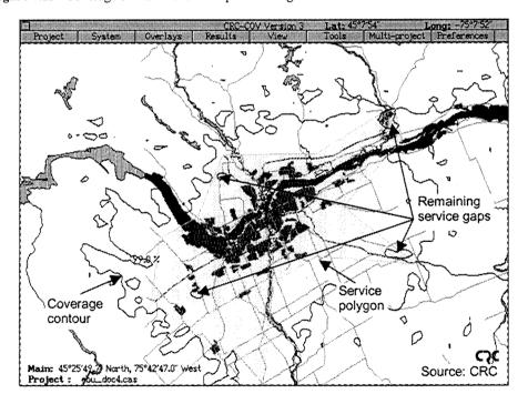
Figure 7.14 Coverage of main transmitter, coverage extender plus two gap fillers
