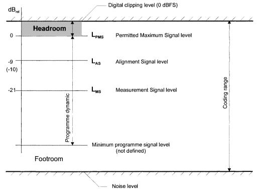
Figure 5.9 Principal level profile of a digital audio broadcast transmission channel
