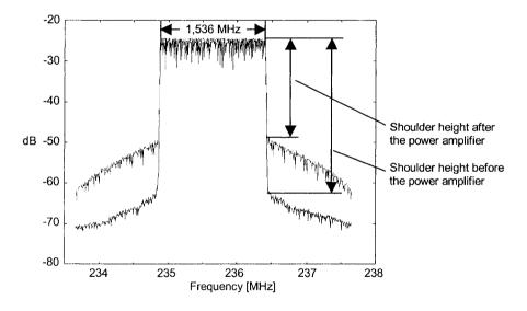
Figure 7.8 Spectrum of DAB signal with amplifier non-linearity
