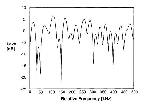
Figure 2.3 Frequency selectivity of multipath fading
