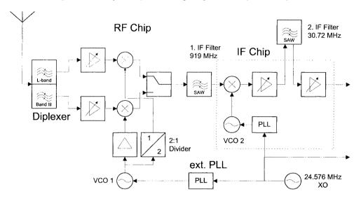
Figure 8.14 Front-end architecture of the D-FIRE chip-set.
