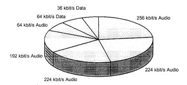
Figure 2.10 An example of how the overall capacity is assigned to individual applications (capacity pie).
