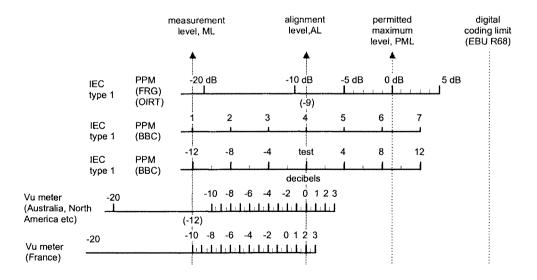
Figure 5.8 Programme level metering, according to (BS.645)
