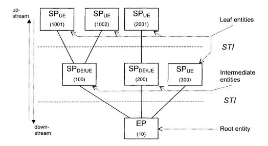
Figure 6.10 Tree-structured DAB collection network (example)
