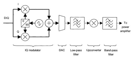
Figure 7.7 Block diagram of DAB transmitter using low IF
