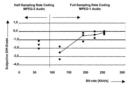
Figure 3.11 MPEG Layer II, stereo
