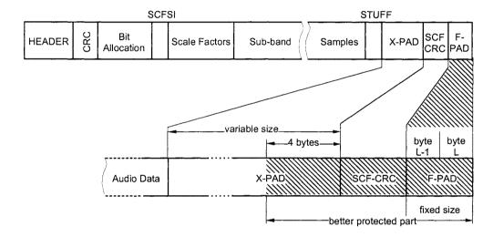
Figure 3.6 Structure of Fixed and Extended Programme-associated Data (F-PAD and X-PAD) and Scale Factor CRC (SCF-CRC) applied to the MSBs of the scale factors for either four or two sub-band groups, depending on the bit rate
