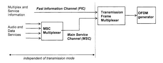
Figure 2.8 Generation of the DAB multiplex
