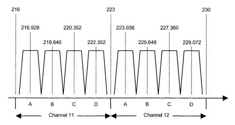
Figure 7.19 Block allocations in Channels 11 and 12 (all frequencies in MHz)
