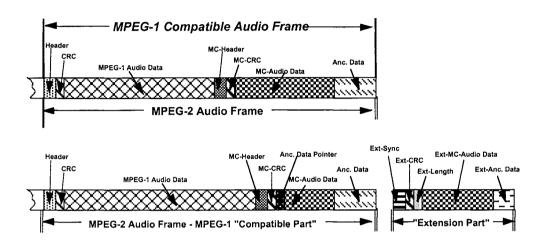
Figure 3.10 ISO/IEC 13818-3 (MPEG-2 Audio) Layer II multichannel audio frame consisting of the MPEG-1 compatible part and the extension part
