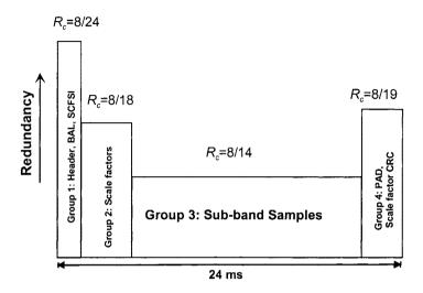
Figure 2.7 Example of an audio UEP profile
