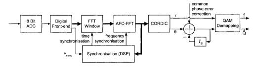
Figure 8.18 D-FIRE OFDM demodulation
