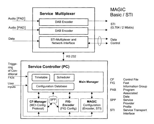
Figure 6.18 STI solution at service provider
