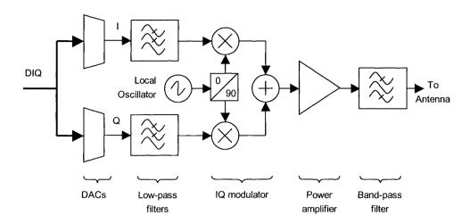
Figure 7.6 Example block diagram of a DAB transmitter with DIQ baseband input
