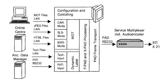
Figure 5.6 PAD inserter
