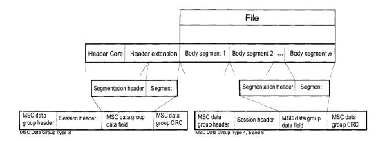
Figure 4.2 Segmentation of an MOT header and an MOT body
