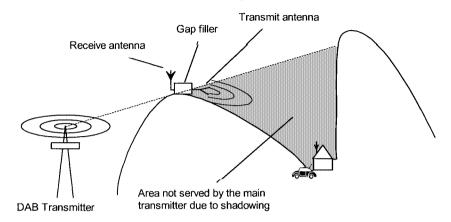
Figure 7.9 Typical application of a DAB gap filler
