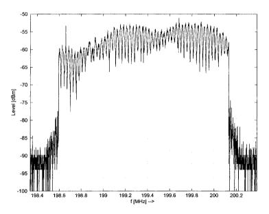
Figure 8.2 DAB signal in frequency domain. Ripple is caused by multipath propagation
