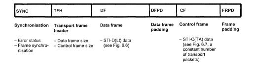
Figure 6.8 Frame structure of the generic transport frame STI(PI,X)
