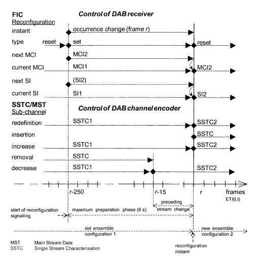
Figure 6.14 Commanding the ensemble reconfiguration via ETI(LI)
