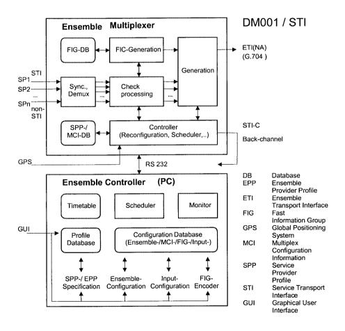
Figure 6.17 STI solution at the ensemble provider
