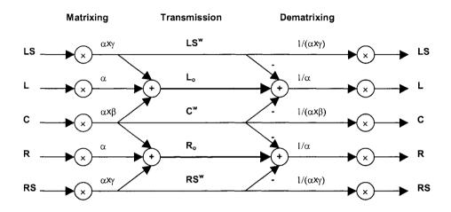
Figure 3.9 Compatibility matrix (encoder) to create the compatible basic stereo signal, and the inverse matrix (decoder) to re-establish the discrete five audio channels
