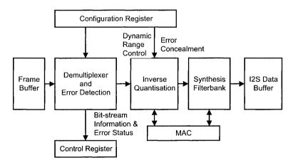
Figure 8.19 Audio decoder block schematic
