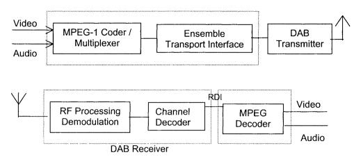
Figure 4.8 Schematic of a DMB system
