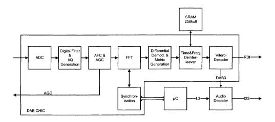
Figure 8.12 JESSI AE-89 DAB Channel Decoder Architecture I - Philips
