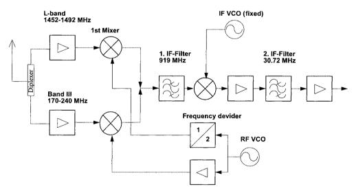
Figure 8.5 Receiver with high-IF for Band III
