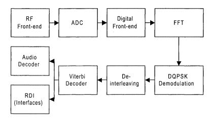
Figure 8.1 Receiver block schematic
