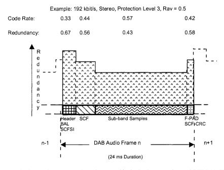
Figure 3.13 Unequal error protection scheme used in the DAB system for an ISO/IEC 11172-3 Layer II audio frame
