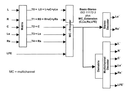
Figure 3.8 Backward compatibility of MPEG-2 Audio with MPEG-1
