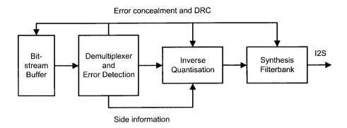
Figure 8.10 Audio decoder block schematic.
