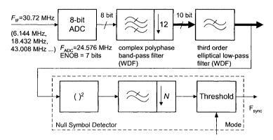
Figure 8.16 D-FIRE digital front-end
