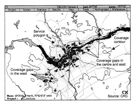
Figure 7.13 Coverage of main transmitter plus coverage extender
