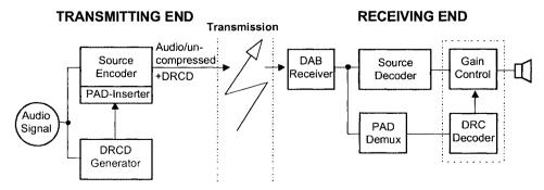
Figure 3.7 Block diagram of a DRC system for DAB
