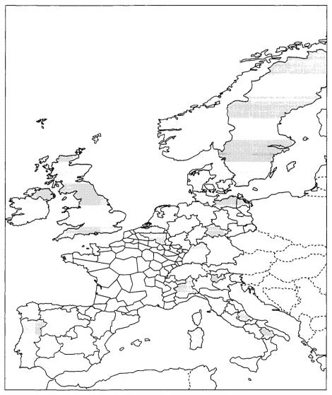
Figure 7.21 Use of Block 12B (first priority) in Europe as agreed at the Wiesbaden Conference in 1995 (shaded areas represent 12B coverage) [© Copyright British Broadcasting Corporation 2000. Reproduced by permission of the British Broadcasting Corporation]
