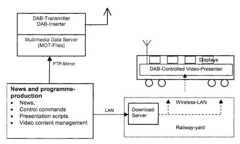
Figure 4.6 Overall structure of the "Mobil-Info" service
