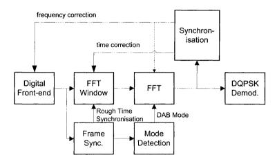
Figure 8.8 OFDM demodulation
