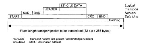
Figure 6.7 Layer structure and format of STI-C(TA) packets
