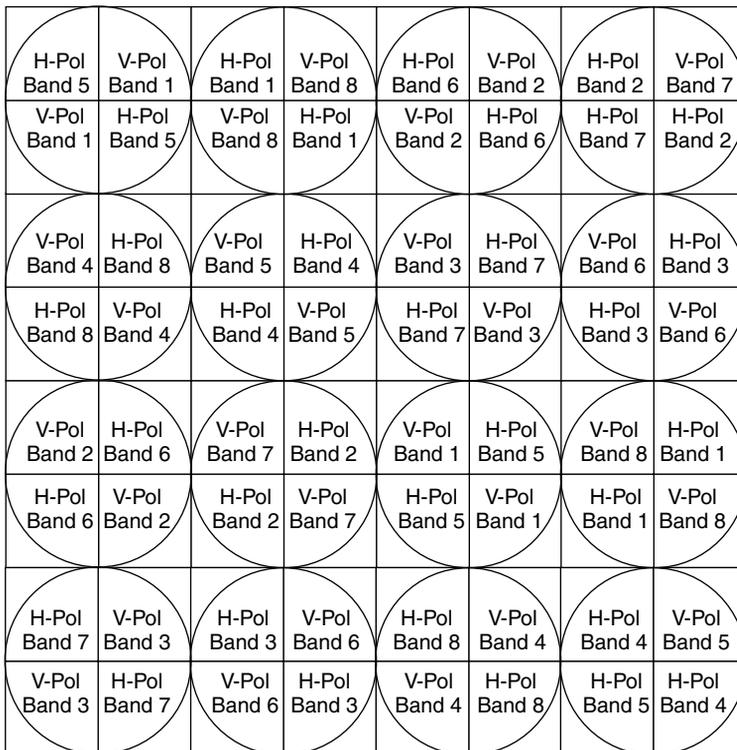
**Figure 12.6** Example of a hub-sector polarization-frequency assignment pattern using 8 frequency sub-bands.
