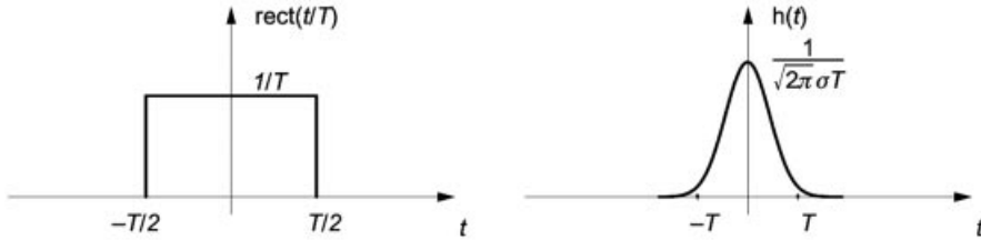
Figure 5.3: Impulse responses for the building blocks of the GSMK transmitter filter
