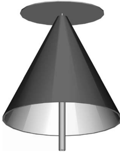
FIGURE 5-32 Discone antenna with coaxial feed with a center conductor connected to the upper disk and a shield connected to the lower cone.
