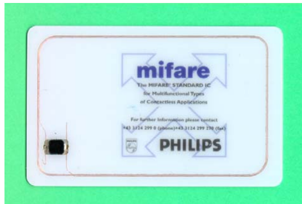
Figure 13.11. Mifare card, showing IC (bottom left) and coil.
