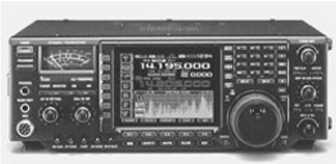
**Figure 6.1** Amateur radio HF transceiver (Courtesy of Waters & Stanton Ltd)
