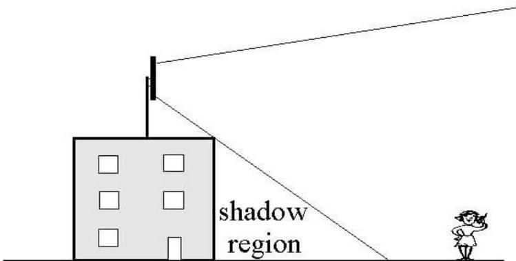
Figure 6.16 Shadowing of coverage from roof-mounted antennas
