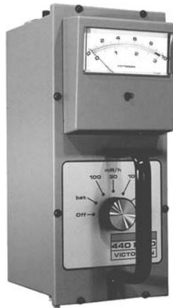
**Figure 8.16** *Victoreen 440RF/D low energy shielded survey meter (Courtesy Victoreen Inc.)*
