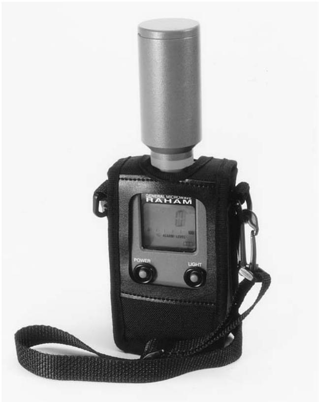
**Figure 7.18** GMC Raham rugged radiation monitor model 2001 (Courtesy General Microwave Corp.)
