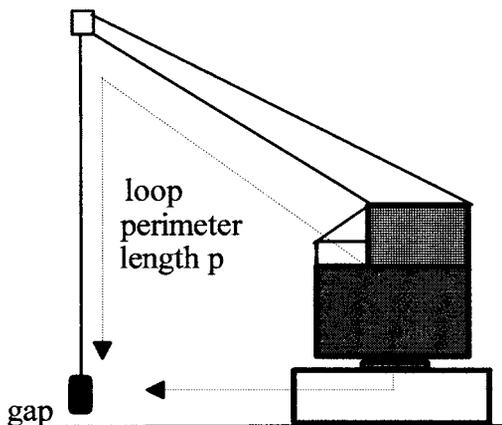
**Figure 4.14** *A crane as a pick-up loop*
