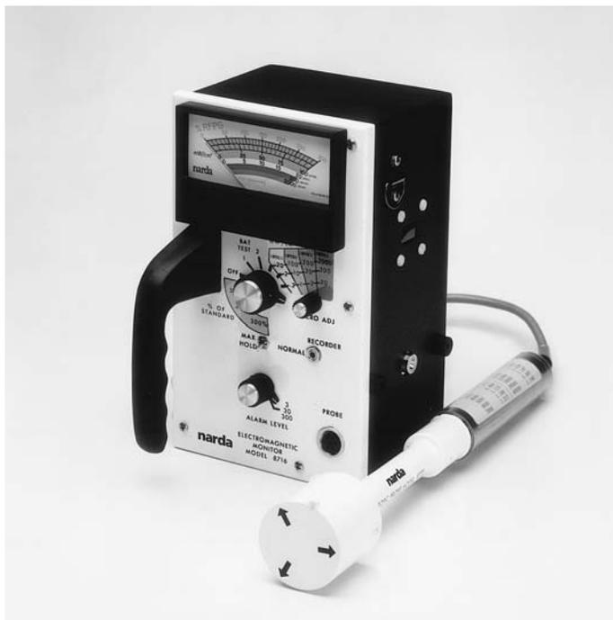
**Figure 7.9** Narda type 8716/8721 analogue RF radiation meter (Courtesy Narda Safety Test Systems)
