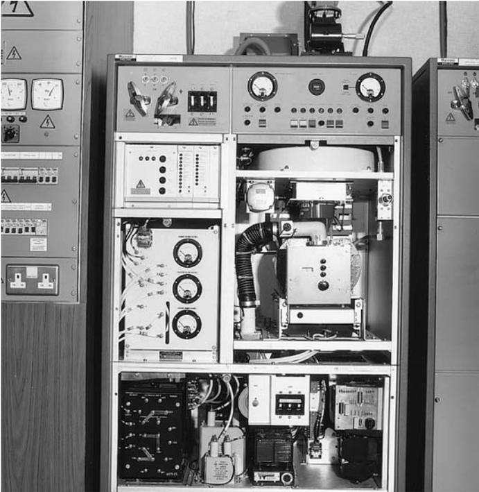
**Figure 2.13** Tactical tropospheric scatter transmitter (Courtesy Marconi Electronic Systems)
