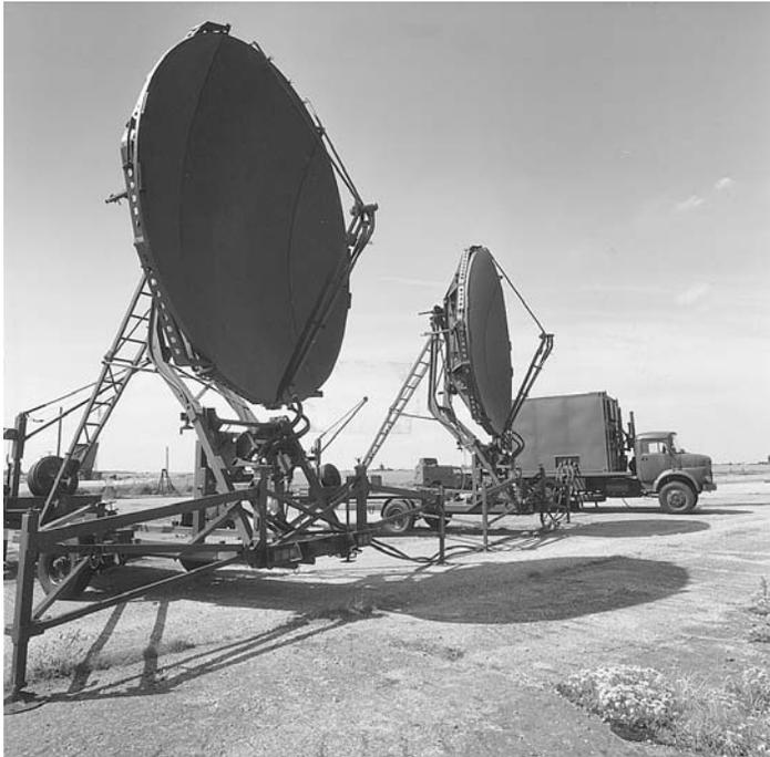
**Figure 2.12** *Tactical tropospheric scatter (Courtesy Marconi Electronic Systems)*
