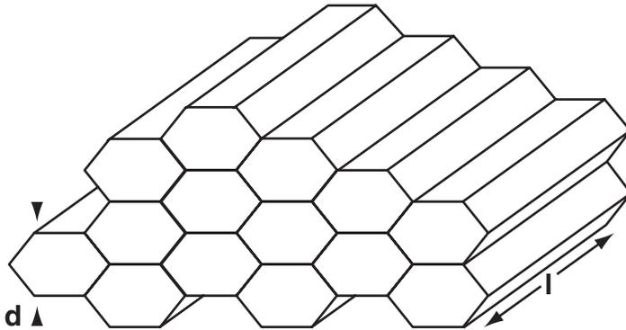
**Figure 11.9** *Honeycomb vent utilising waveguides below cut-off*
