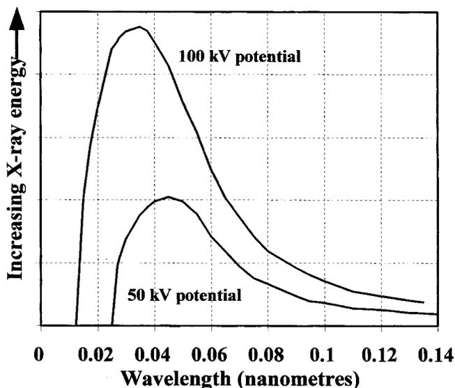
**Figure 8.3** X-ray energy distribution versus tube voltage
