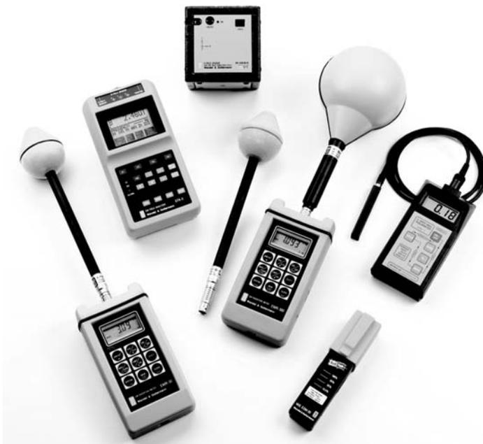
**Figure 7.13** Grouping of NSTS (W&G) instruments (Courtesy Narda Safety Test Systems)
