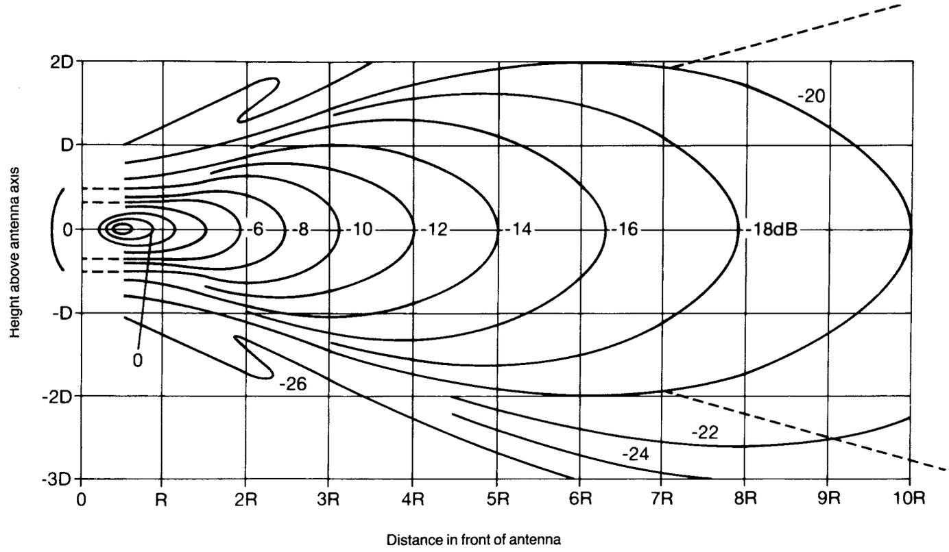
Figure 5.4 Far field of circular aperture antennas
