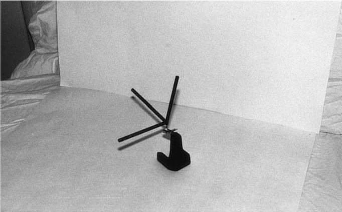
**Figure 7.3** *Sensor isotropic antennas – electric field*
