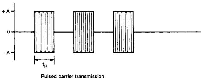
**Figure 1.7** *Pulse modulation*
