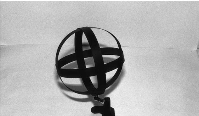
**Figure 7.4** *Sensor isotropic antennas – magnetic field*
