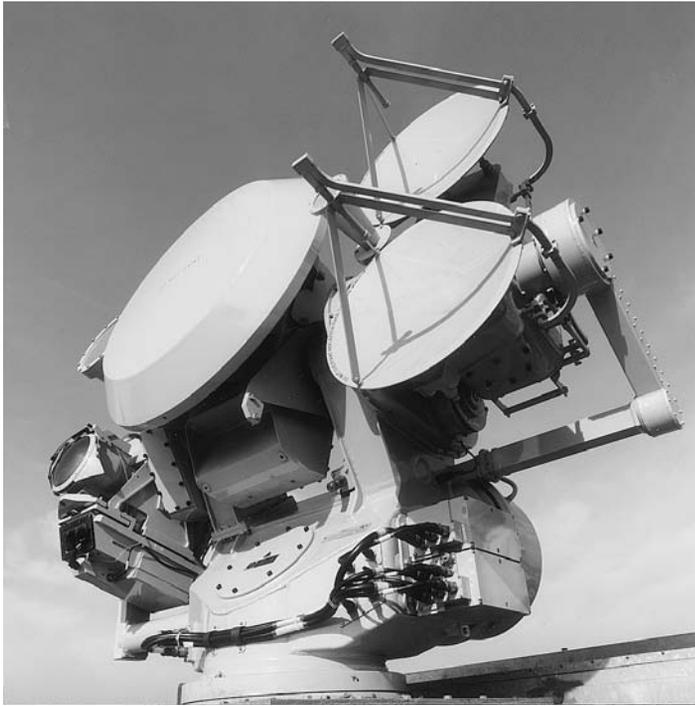
**Figure 2.21** *Seawolf tracker radar and gunfire control system (Courtesy Alenia – Marconi)*
