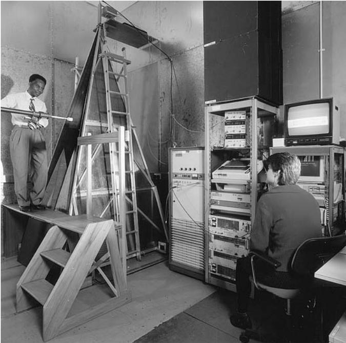
**Figure 12.3** NPL tapered TEM cell for calibration in the range 180 MHz to 2.4 GHz
