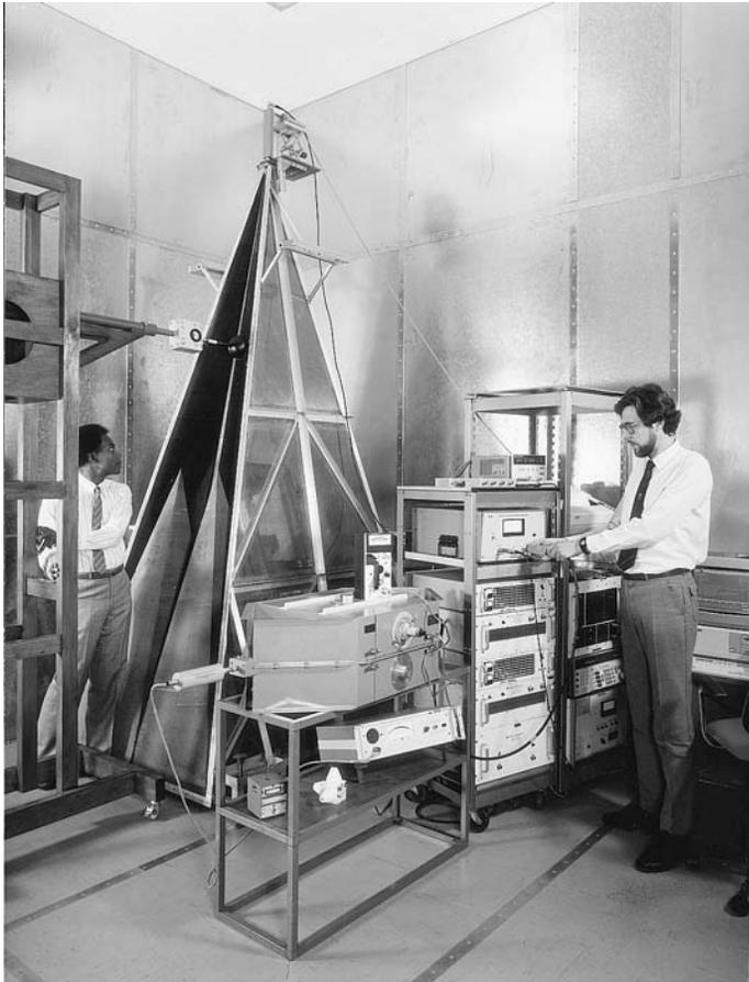
**Figure 12.2** TEM cells used for calibration in the range 3 kHz to 2.4 GHz
