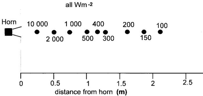
**Figure 10.16** Axis power density calculation for Figure 10.15
