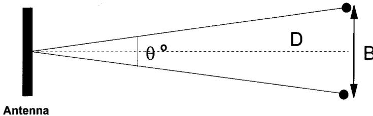
Figure 10.7 Beamwidth approximation by measurement
