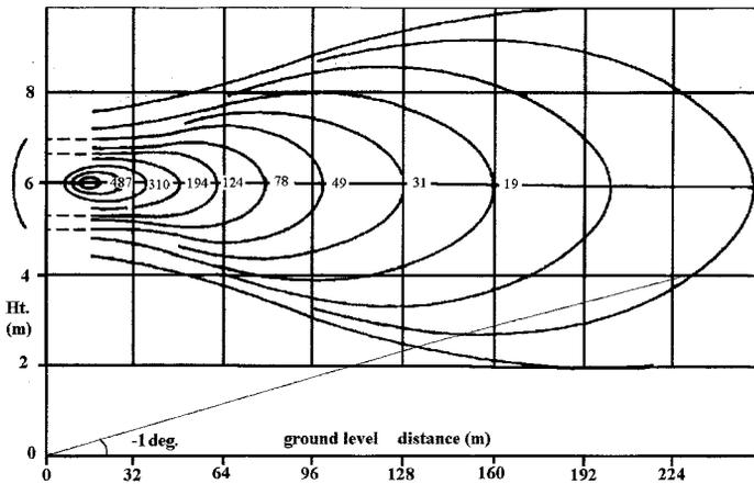
**Figure 10.8** *Change of beam elevation on calculation diagrams*
