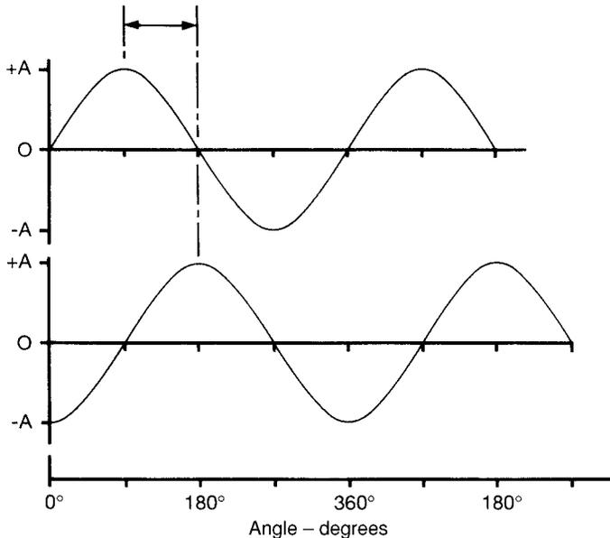
**Figure 1.3** *Phase difference between two waveforms*
