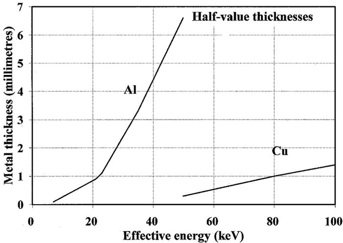
**Figure 11.4** Half value layer thicknesses plotted from Table 10.1
