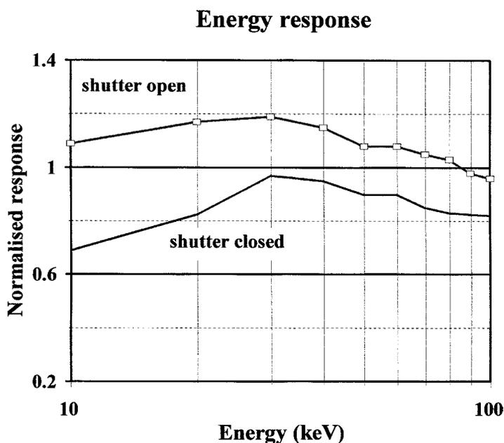
**Figure 8.19** *SmartION energy response curve (Courtesy Mini-Instruments Ltd)*
