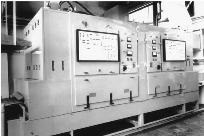
**Figure 2.22** Strayfield 100 kW post-baking unit (Courtesy Strayfield International)
