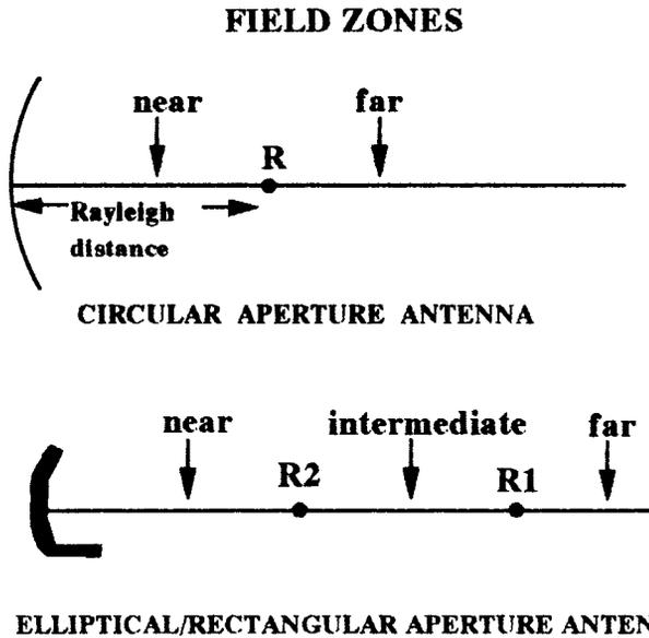
**Figure 5.3** Radiation field zones of antennas
