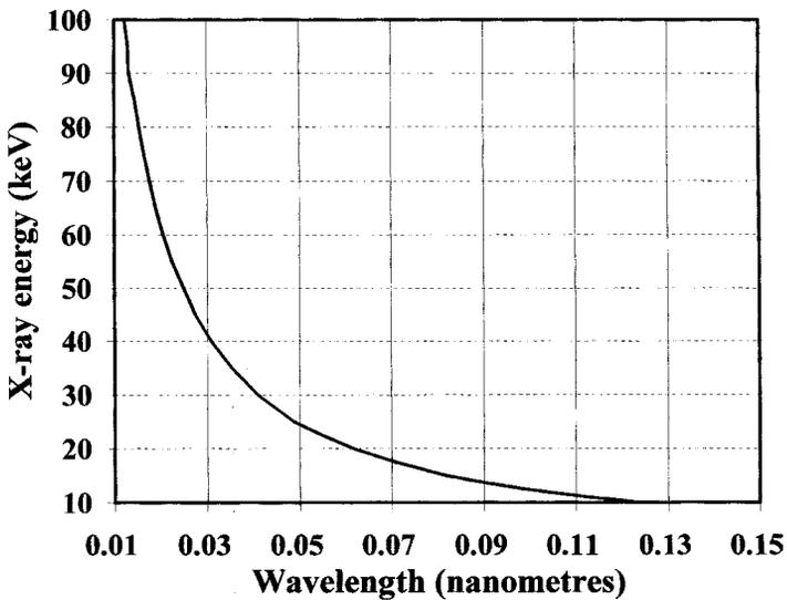
**Figure 8.2** *X-ray wavelength versus X-ray energy (keV)*
