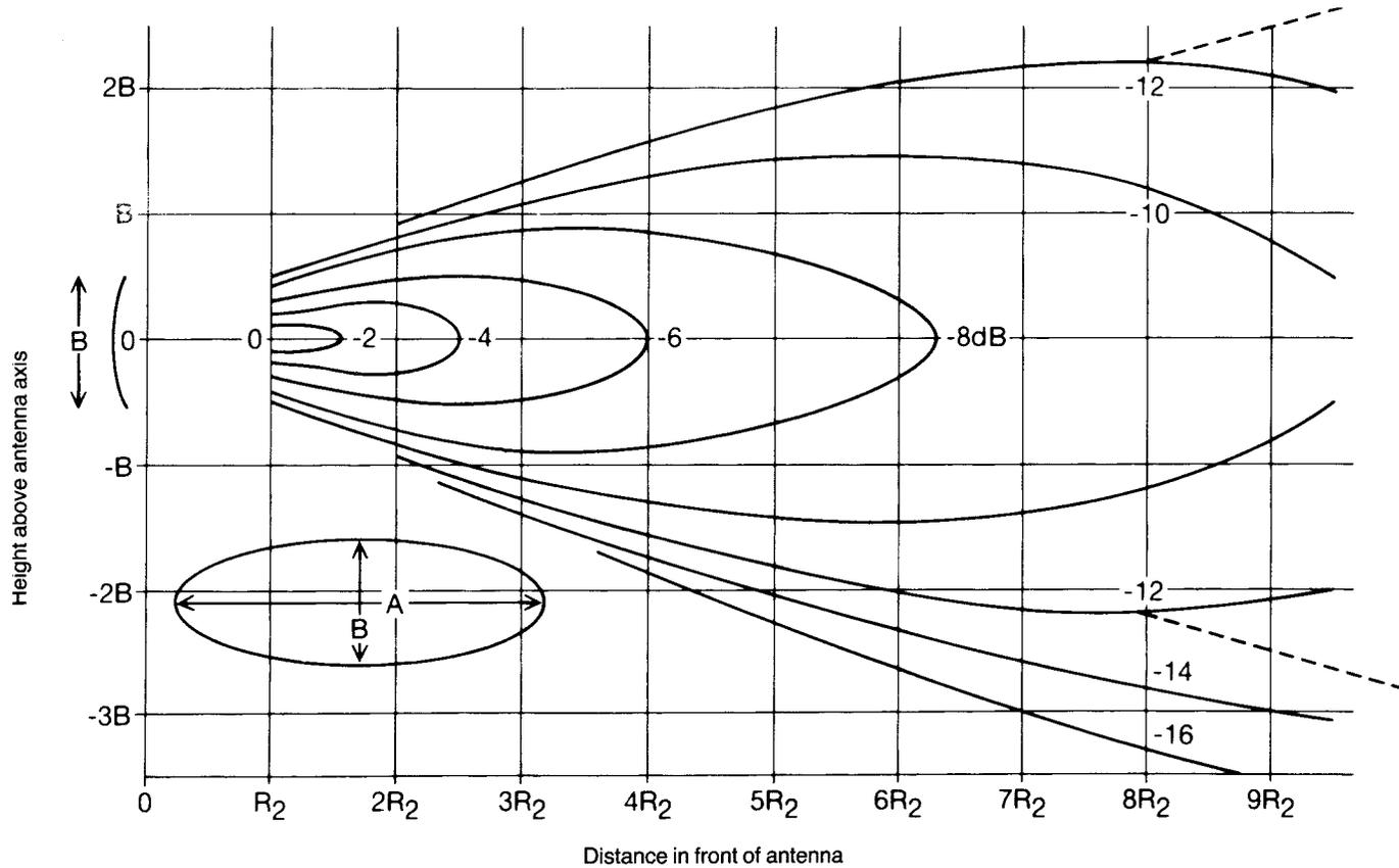
**Figure 5.5** Elliptical and rectangular aperture antennas – intermediate field with larger aperture dimension horizontal
