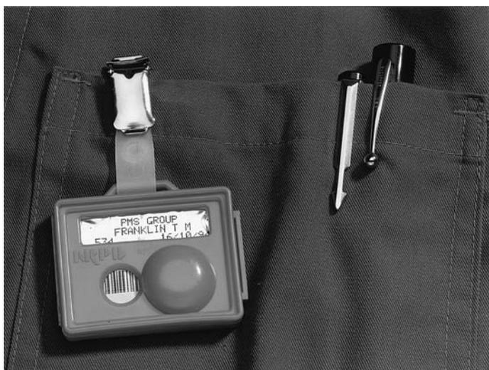
**Figure 8.13** *Thermo-luminescent dosimeter (TLD) (Courtesy NRPB)*
