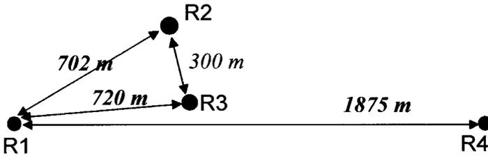
Figure 10.10 Typical airport radar layout in plan view
