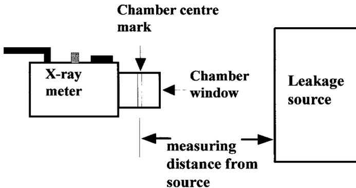
**Figure 8.20** *Measurement distance measurement for ionising chamber instruments*
