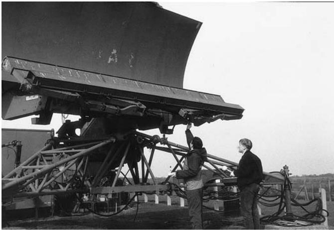
**Figure 10.3** *RF leakage measurement on radar waveguides during training*
