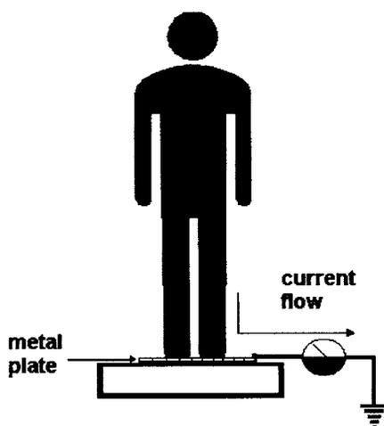
**Figure 3.4** *Limb current measurement concept*
