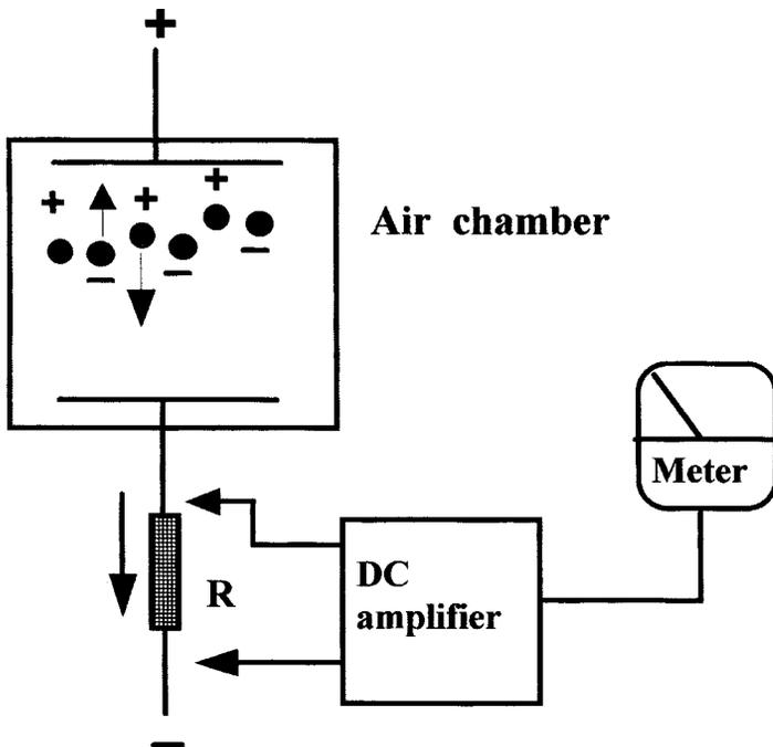
**Figure 8.11** Ionisation chamber X-ray measuring instrument – basic concept
