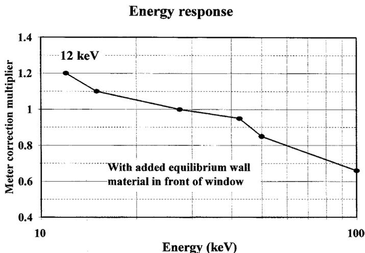
**Figure 8.17** *Victoreen 440RF/D energy response (Courtesy Victoreen Inc.)*
