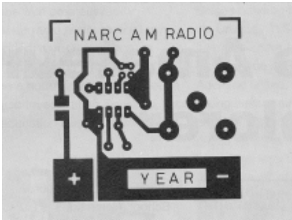
Figure 2a The PCB, solder side
