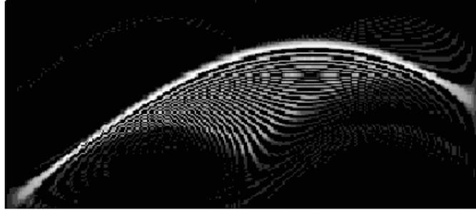
**Fig. 10.13.** An example of the presence of cross-terms in the WVD. The original signal is a chirp, first rising in frequency and then falling. High-energy coefficients appear beneath the main arc of energy in the transform plane, yet the time-domain signal contains no such tones. Higher-level interpretation routines are beset with the problem of separating such artifacts from genuine features of the signal's time evolution.
