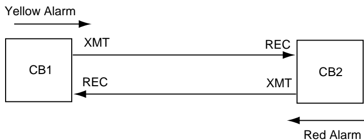
Figure 15.13 T1 alarm generation example. A red alarm is produced by a receiver to indicate it has lost frame alignment, and a yellow alarm is returned to a transmitting terminal to report a loss of some alignment at the receiving terminal
