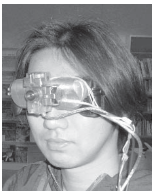
Figure 4. A wearable camera, display, and two mono-axis gyro sensors
