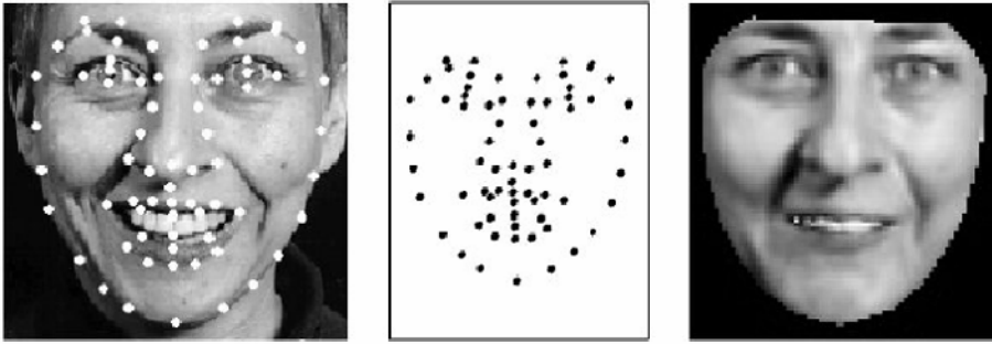
Figure 3. The training image is split into shape and shape-normalized texture (Cootes et al., 2001)
