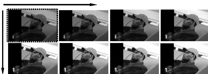
Figure 8. An example of a video sequence of fading in (the frame with dotted border is shot cut detected by the proposed method)
