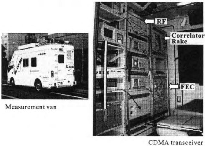
Figure 12.16 Measurement van equipped with W-CDMA transceiver.
