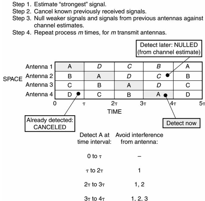
continues, with the known signals cancelled and the new signals nulled on the basis of channel characteristics.
