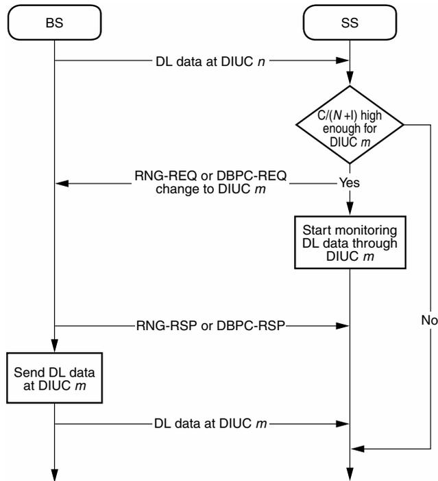
bandwidth stolen from a lower QoS connection. The SS could also use some of the bandwidth to react more quickly to changing environmental conditions by sending, for instance, a DBPC-REQ message.
