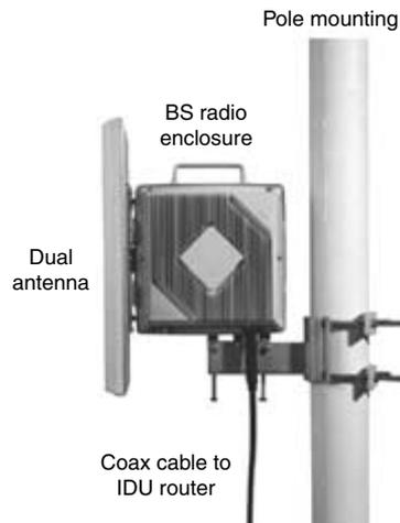
a pole, a tower, or a wall. The remote station ODU is an unprotected unit, where a single transceiver with a medium-power amplifier is used. The enclosure is directly connected to the flat-panel antenna. In addition, an alignment indication connector is also provided for antenna installation and alignment with the base station.
