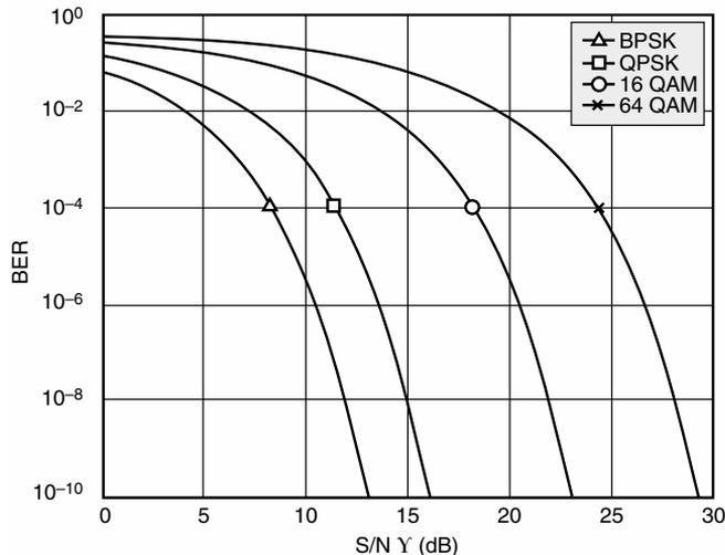
and 64 QAM.<sup>1</sup> The set of adaptation/switching thresholds is then obtained by reading the  $S/N$  points corresponding to a target BER. For example, if the target BER is  $10^{-4}$ , the thresholds are 8.4, 11.4, 18.2, and 24.3 dB, respectively (as indicated by the markers on the figure).
