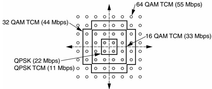
D0, D1, . . . , D7, which are generated by applying a set-partitioning rule to the signal constellations shown in Fig. 22-3. Each subset contains 2, 4, and 8 symbols for 16/32/64 QAM constellations, respectively. The remaining higher-order bits (1, 2, and 3 bits for 16/32/64 QAM, respectively) select one of the symbols from each subset. In the QPSK TCM mode, the lower-order 2 bits select one of the four subsets, D0, . . . , D3,
