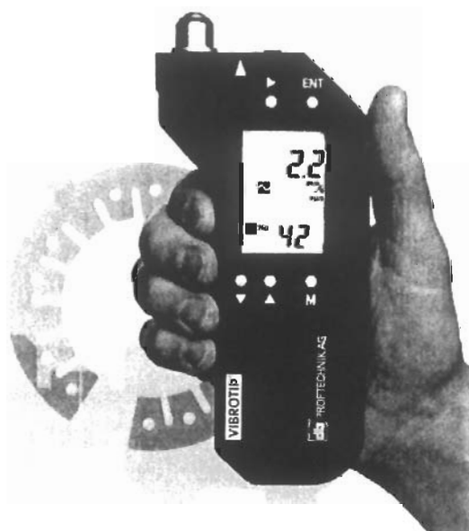
Figure 11-28. Portable instrument used to monitor pump condition. (Courtesy of Prueftechnik AG, D-85730 Ismaning, Germany.)
