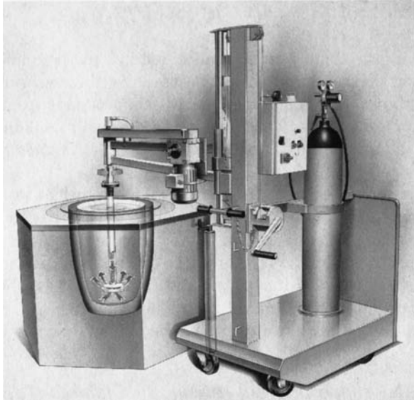
Figure 6.2 The Foseco Mobile Degassing Unit.
