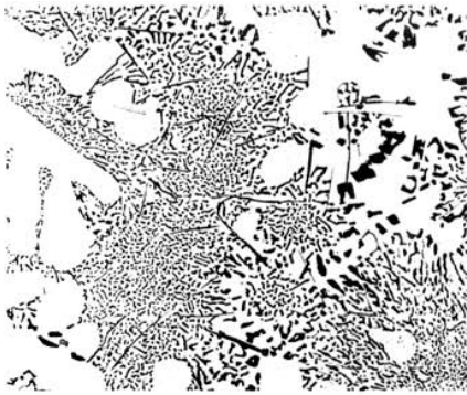
LM6 before modification
