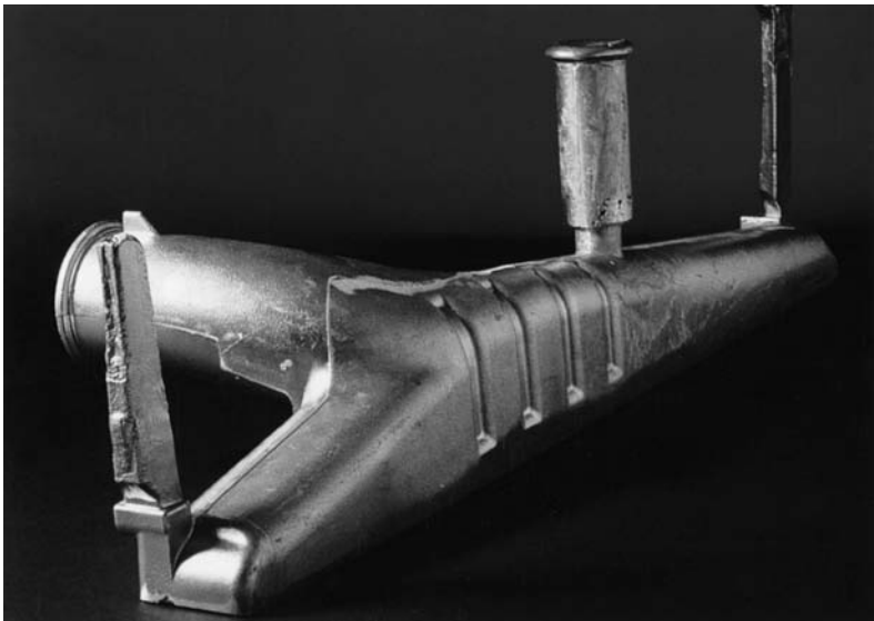
Figure 8.8 Gravity diecast casting directly cast through a SIVEX FC filter.
