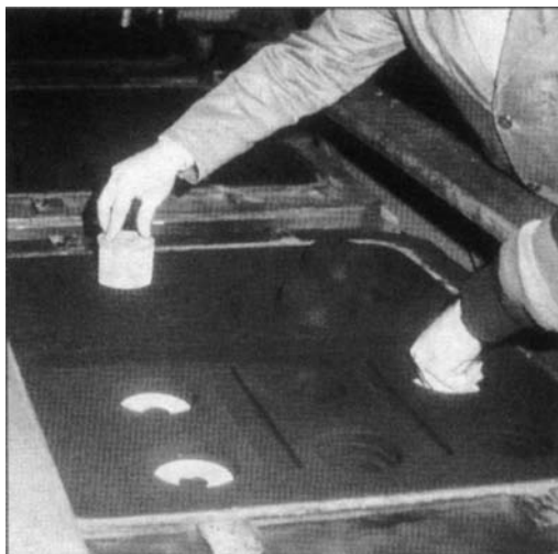
Figure 17.11 The KALSERT system in operation. KALMINEX sleeves being inserted into green sand moulds on an automatic moulding line.
