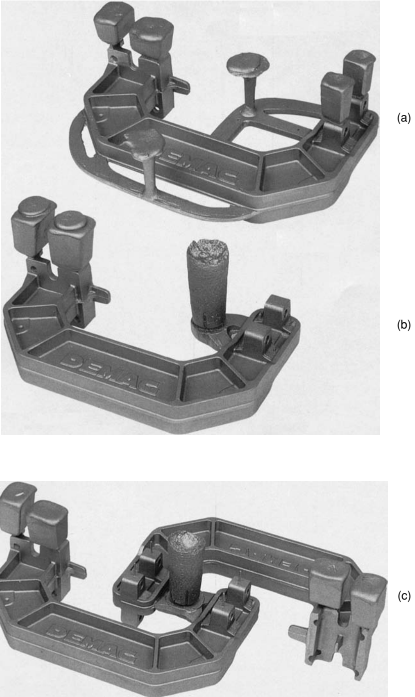
Figure 8.7 (a) Sand cast aluminium casting using standard running system. (b) Casting made using the KALPUR direct pouring sleeve/filter unit. (c) Optimised direct pouring system.
