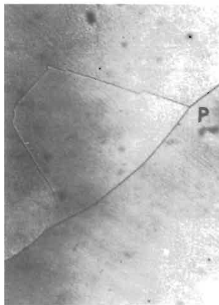
Fig. 55. Annealing twin in an iron–aluminum alloy after prolonged grain growth. 170 \times . (After CAHN and COLL [1961].
