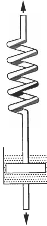
Fig. 48. A Maxwell element describing viscoelasticity. The spring represents the rubber modulus, and the dashpot the viscosity. The dashpot becomes 'stiffer' with decreasing temperature and/or increasing molecular weight. For a chemically crosslinked rubber it will be locked solid.
