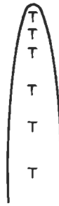
Fig. 17. Near the tip of an elastic crack, the opening is parabolic (see eq. 15). This opening can be made equivalent to the displacement of a distribution of prismatic dislocations as shown. The stress and displacement outside the crack is then given by a distribution of “crack dislocations”.
