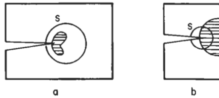
Fig. 16. The path for calculating J in (a) can be shrunk from a position where the crack and the shaded deformation zone are fully enclosed to any arbitrary size. In (b) there is no position of S enclosing the crack, which runs entirely through elastic material.
