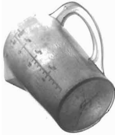
Fig. 34. Crazes in an injection-moulded polymer jug.
