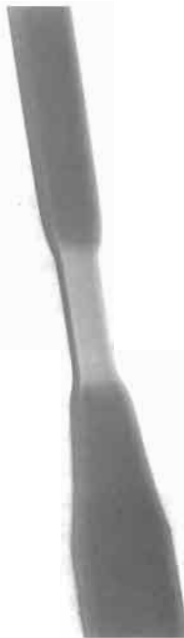
Fig. 26. A polymer sample which has been partially drawn.
