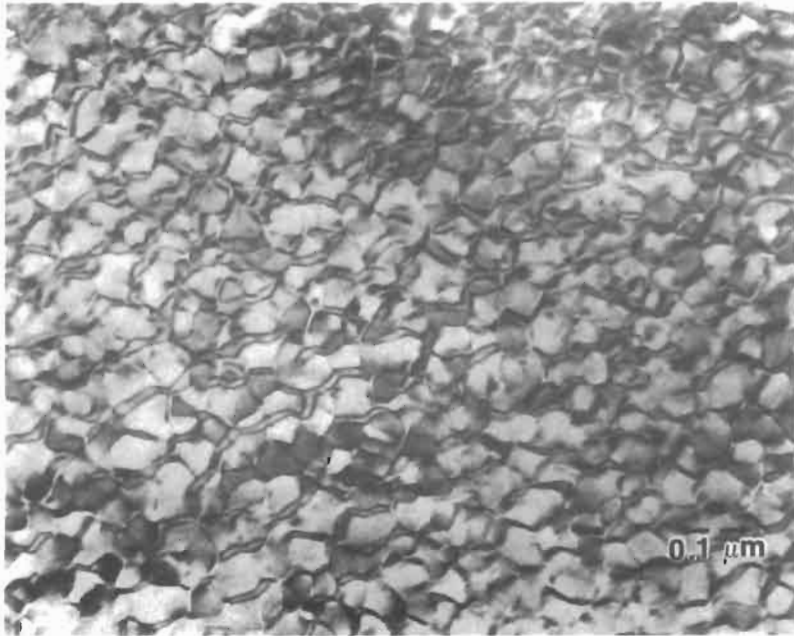
Fig. 9. Transmission electron micrograph of cellular precipitation structure within single-grain-sintered Co-Cu-Fe-Sm aged to peak coercivity ( 560 \text{ kA/m} = 7 \text{ kOe} ). Section normal to easy magnetic axis (hexagonal axis). Cell interiors have 17-2 structure, cell boundaries have 5-1 structure, fully coherent. Coercivity controlled by domain-wall pinning by cell boundaries. (From LIVINGSTON and MARTIN [1977].)
