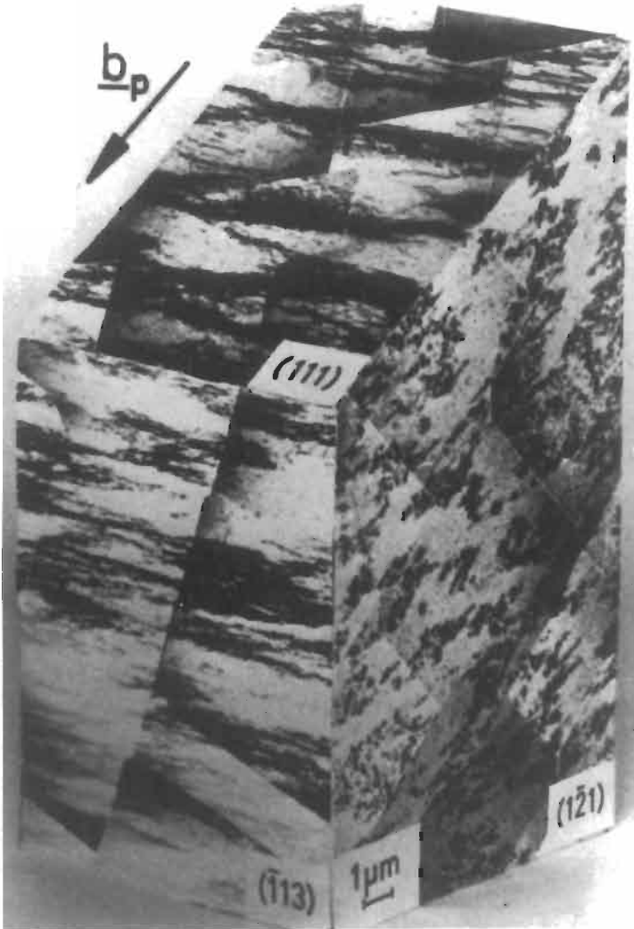
Fig. 6. The formation of dislocation dipoles by (a) and (b) mutual trapping of edge dislocations, and (c) a double cross-slip mechanism. (d) The clumping of these dipoles forms loop patches seen in a three dimensional view corresponding to region A of the CSSC (plastic shear strain amplitude, 2.6 \times 10^{-3} , shear stress = 19.8 MPa) from the unpublished work of Ackermann and Mughrabi via LAIRD et al. [1986].
