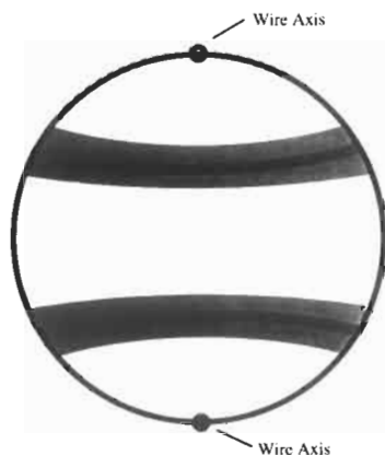
Fig. 7. A pole figure drawn for the \{100\} planes of drawn aluminium wire. The dark bands on the stereogram represent orientations of high probability of the plane normals for the 111 wire texture. The wire axis corresponds to the top and bottom poles of the stereogram.
