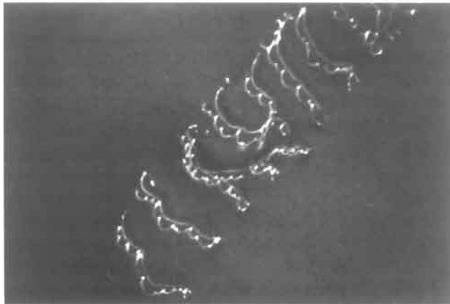
Fig. 25. Weak-beam electron micrograph of single crystal Nimonic PE 16 foil ( \text{Ni}_{42}\text{Fe}_{33}\text{Cr}_{18}\text{Mo}_2\text{Al}_3\text{Ti}_2 ). Dispersion of \gamma' -particles with r=8 nm (invisible), f=0.09 , glide plane (111), tensile axis [\bar{1}23] (NEMBACH and NEITE [1985]). 45000 \times .
