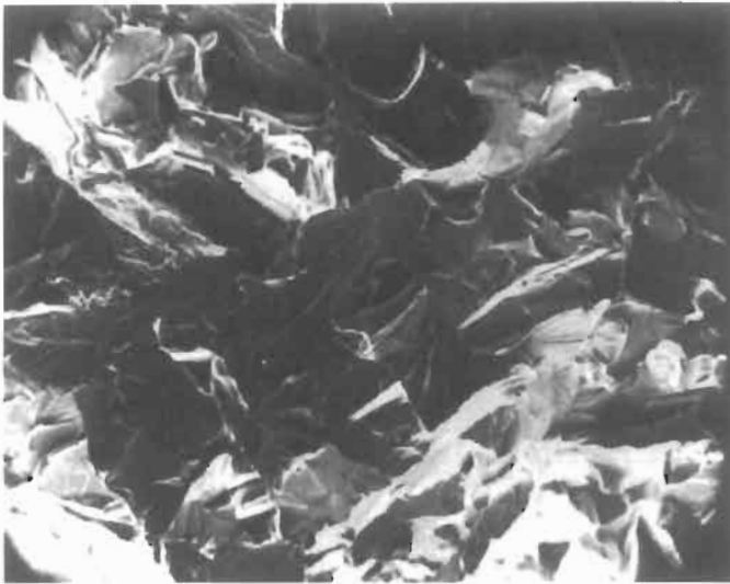
Fig. 10. Appearance of relatively brittle fracture in steel. Top: the fracture is along the grain boundaries (intergranular). Bottom: the fracture is transgranular. (Courtesy C. INTERRANTE.)
