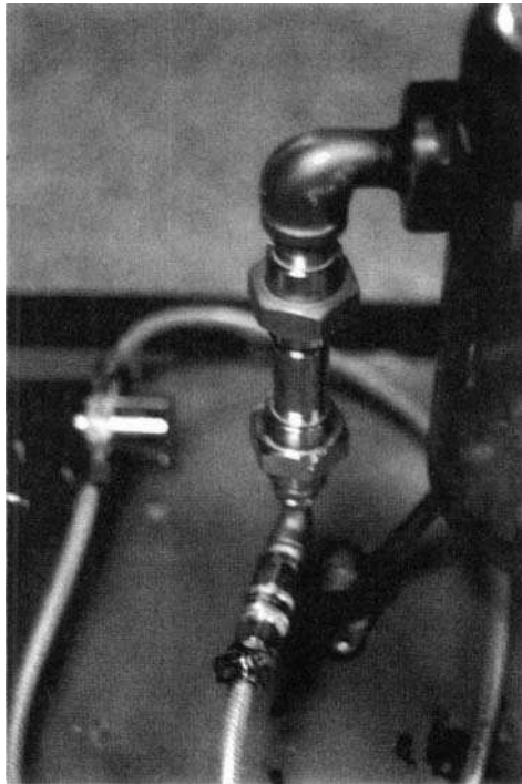
Figure 10. The catalyst chamber of the H_2 generator shown in Figure 8. The chamber is 3 inches long and \frac{3}{4} inches in diameter. It contains less than 5 grams of catalyst, enough to supply sufficient H_2 to run the engine.
