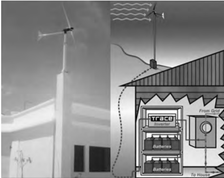
FIGURE 5.6 Building-integrated wind power. (From http://www.oksolar.com/wind/ . With permission.)
