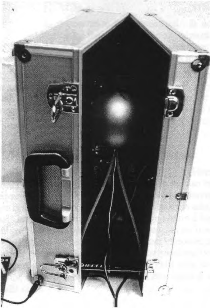
Fig. 9: Transmitter and frequency generator in the aluminum suit-case (problematic operation!)
