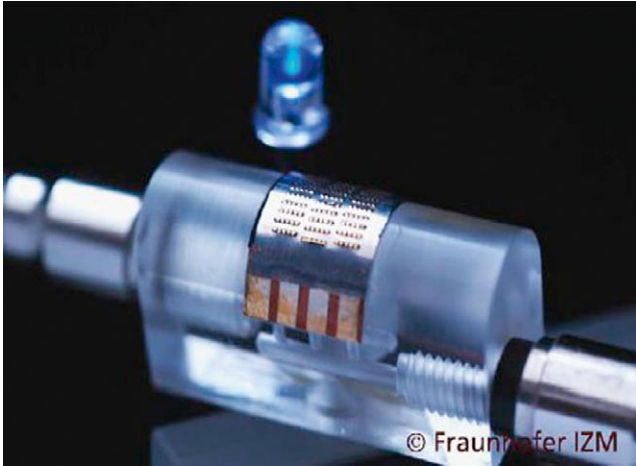
FIGURE 2.12 Fraunhofer IZM prototype of miniature fuel cell powering a LED, after [28].
