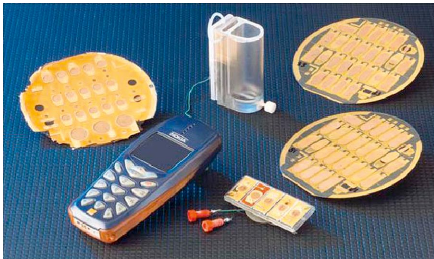
FIGURE 2.23 From the wafer to the phone, fuel cells from the CEA, after [77].
