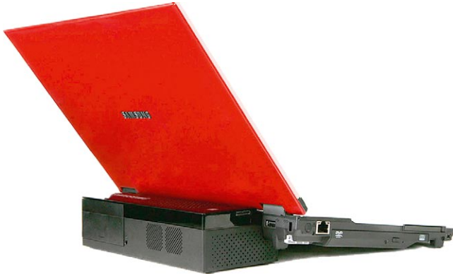
FIGURE 2.25 Samsung DMFC prototype for laptop computer, presented in August 2007.
