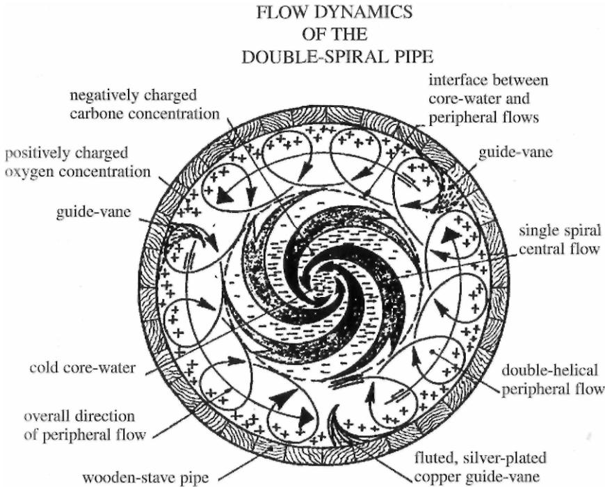
Fig. 16: Pipe cross-section showing double spiral flows<sup>6</sup>
