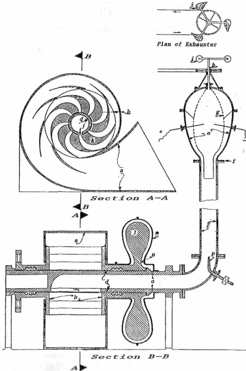
Fig. 19: Air-turbine diagram - patent No. 145141
