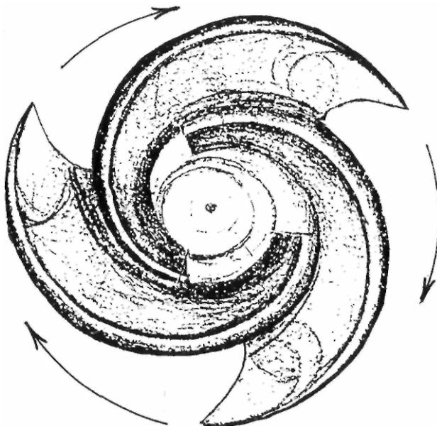
Fig. 11: 3-blade Bio-impeller
