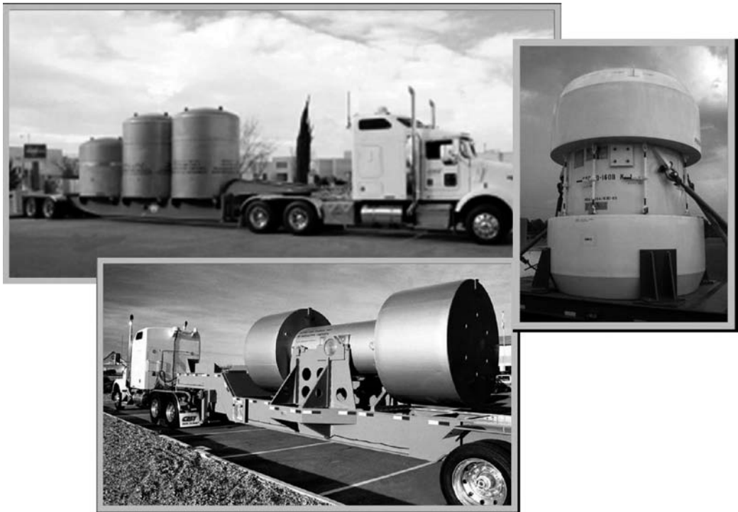
FIGURE 12.6 NRC licensed packagings for transportation of TRU waste.
