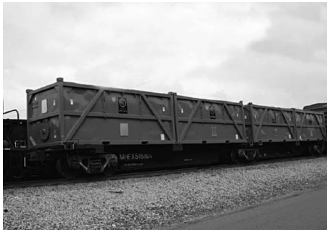
FIGURE 13.2 Four Type A 7A shielded bulk intermodal containers on a 177 ton capacity railcar ( http://www.mhfls.com/main/transpost.asp ).
