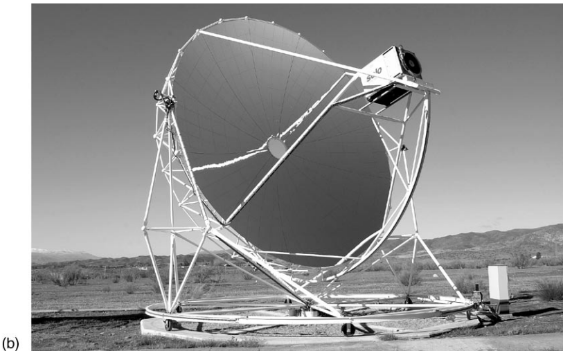
FIGURE 3.20 Parabolic dish collector. (a) Schematic diagram. (b) Photo of a Eurodish collector (from www.psa.es/webeng/instalaciones/discos.html ).
