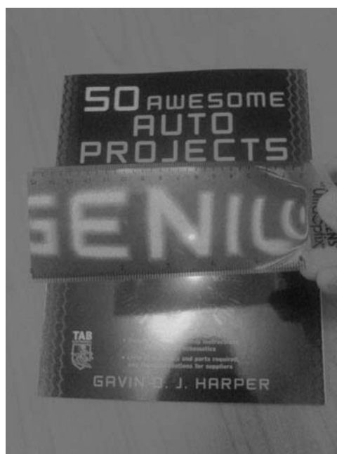
Figure 8-20 A thin Fresnel lens shown magnifying.
