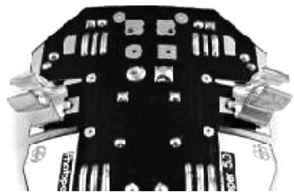
Figure 16-14 Both motor mounts ready. Image courtesy Solarbotics.
