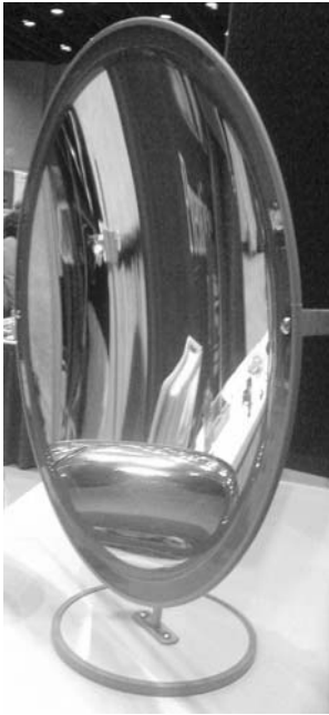
Figure 8-12a and b Parabolic mirrors take incoming parallel light (from the sun) and focus it to a point.
