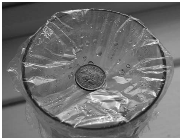
Figure 7-3 Precipitated water in the demonstration still.
