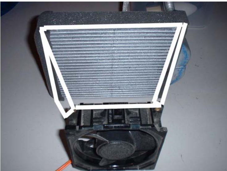
Make a duct (box) between the fan and the heater core with cardboard, hard plastic or plastic sheeting or wood to force all of the air through all of the heater core.
