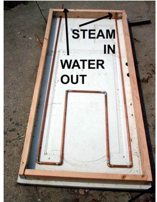
Copper pipes and wood under the black plastic and glass
