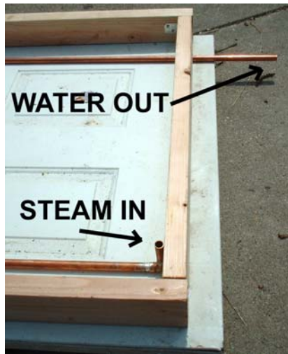
Close up of the Steam In and Water Out
