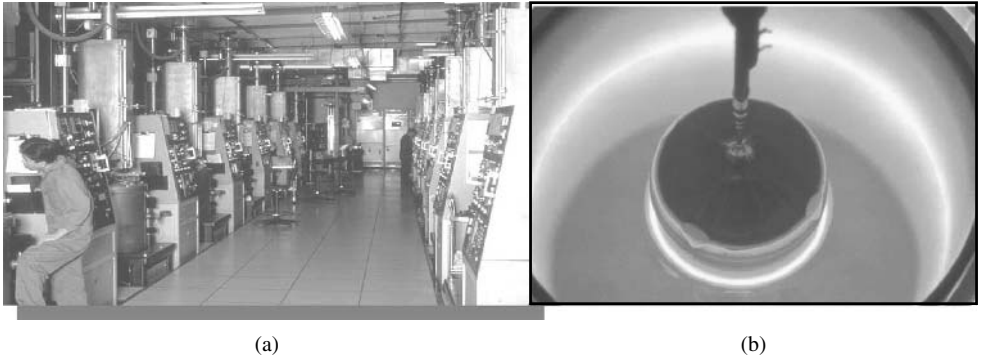
Figure 6.1 Cz pullers in a PV-production environment (a) and growing Cz crystal (b) in a quartz crucible
