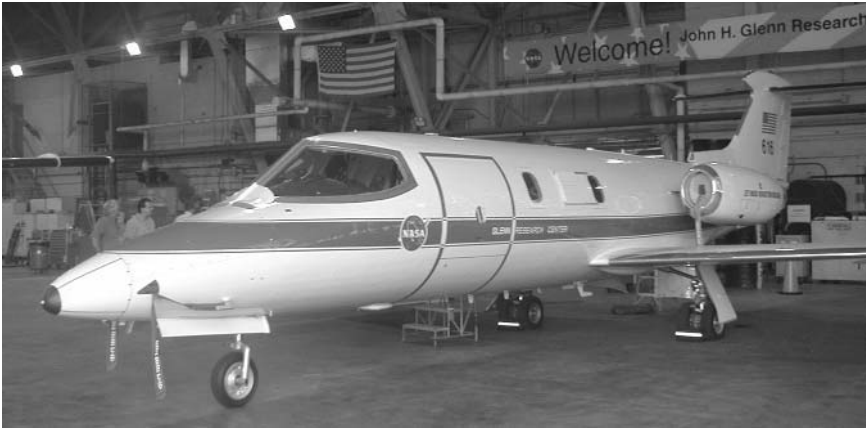
Figure 10.7 The NASA Glenn Research solar cell calibration aircraft. (Photo courtesy of NASA)
