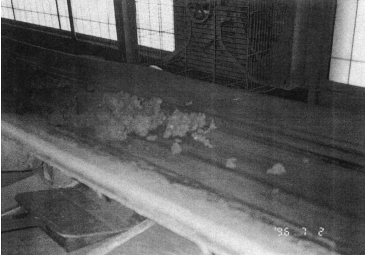
Photo 25.2 Sludge entering furnace.
