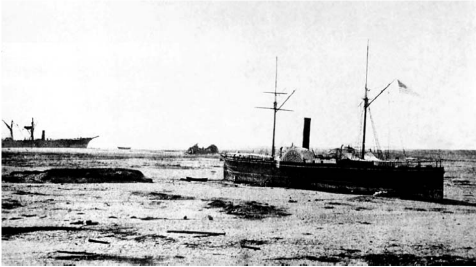
Figure 2.11. The American warship Wateree in the foreground and the Peruvian warship America in the background. Both ships were carried inland 3 km by a 21 m high tsunami wave during the Arica, South American event of August 13, 1868. Retreat of the sea from the coast preceded the wave, bottoming both boats. The Wateree , being flat hulled, bottomed upright and then surfed the crest of the tsunami wave. The America , being keel-shaped, was rolled repeatedly by the tsunami. Photograph courtesy of the United States Geological Survey. Source: Catalogue of Disasters #A68H08-002.
