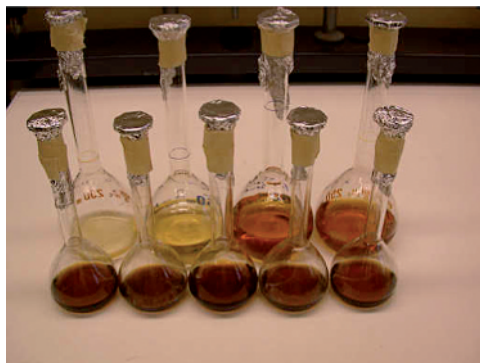
Figure 7. The raw extraction of quinolizidine alkaloids from different lupine species in the Research and Teaching Laboratory of Applied Botany of the University of Joensuu (Photo: T. Aniszewski). Observe the different colours of the raw extracts, which signifies different concentrations of alkaloids in different species.
