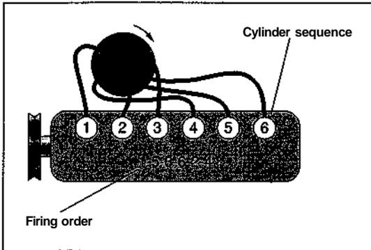
✓ Vehicles with front-wheel drive have transverse engines, usually combined with the transmission into a single unit called a transaxle. On these engines, the cylinders run from one side of the car toward the other, with the #1 cylinder on the passenger side of the vehicle. (See Figure 12-4.)
