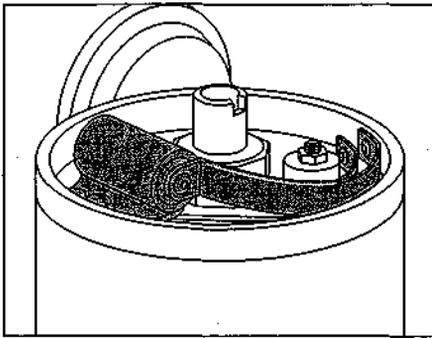
4. Use a clean, lint-free rag to wipe around the breaker plate where the condenser was resting. Then take the new condenser and slide it in where the old one was.
