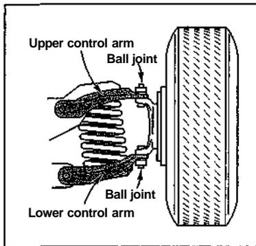
The steering linkage actually connects to the wheels, which are held in place by a spindle that goes through the wheel and is attached to upper and lower control arms (refer to Figure 11-2). The control arms allow the wheels to turn in any direction. To keep things moving freely, ball joints are located at the points on the control arms where the movement takes place.
