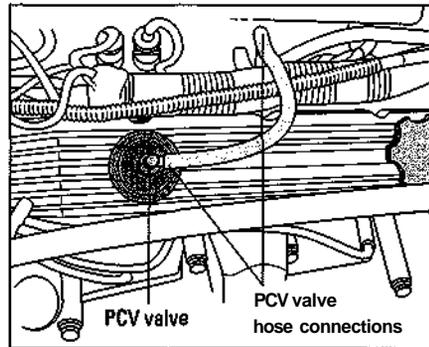
**✓ If your engine is carbureted,** look for a  $\frac{1}{8}$ -inch diameter hose that leads from the bottom area of the carburetor to the top of the valve cover or to the oil filler hole (see Figure 13-7). If your engine has *both*, you want the hose that does *not* lead to the oil filler hole.
