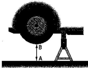
1. Measure the distance from the ground (A) to the bottom of the tire (B) while the car is jacked up.
