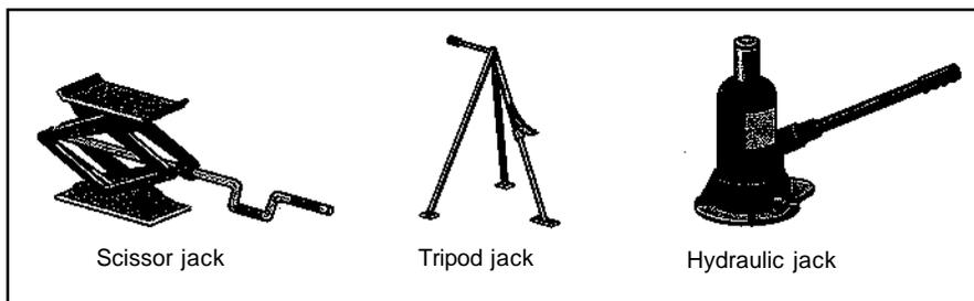
4. If you have jack stands, place them under the car, near the place where the jack is touching the vehicle (see Figure 1-2). Raise the stands until they are high enough to just fit under, and lock them in place. Lower the jack until the car is resting on the jack stands. Then remove the jack.
