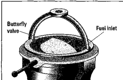
If your car has a *manual* choke (as opposed to an automatic choke), see whether the butterfly valve opens and closes when someone pushes the choke knob on the dashboard in and out.
