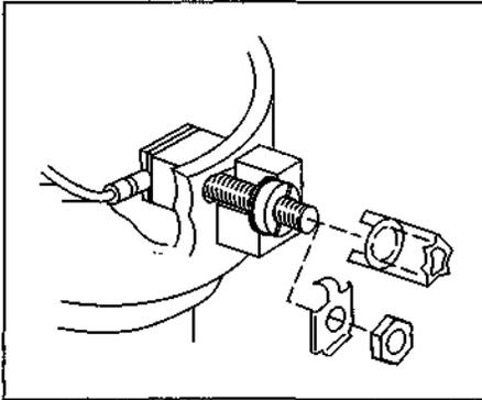
**Figure 12-23:** On other distributors, the nut on the primary terminal must be loosened to release the contact spring and lead wires.
