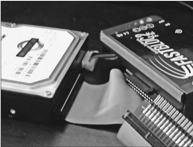
Figure 6-11: Data cable and power cable connected to the acquisition hard drive.
