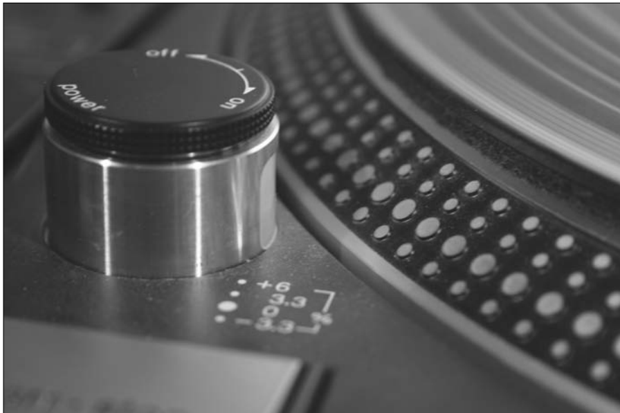
Figure 4-1: The power switch on a turntable, with the strobe light underneath it shining onto the calibration dots on the deckplatter.
