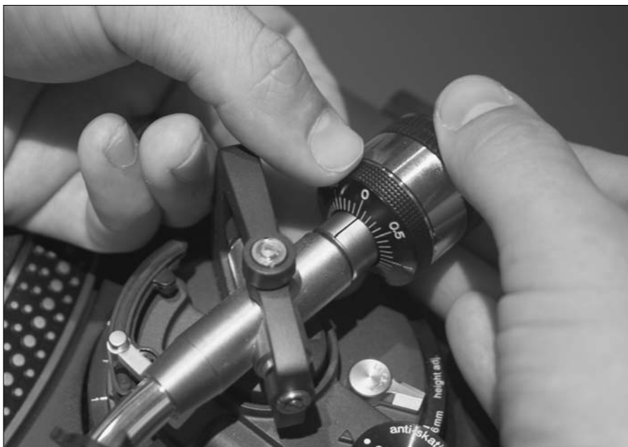
Figure 11-4: One hand supports the back of the counterweight, while the other rotates only the numbered ring.
