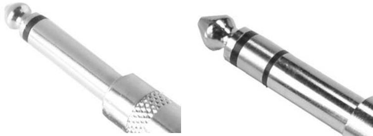
Figure 11-2: Left: A mono quarter-inch jack (TRS) connector. Right: A stereo quarter-inch jack connector.
