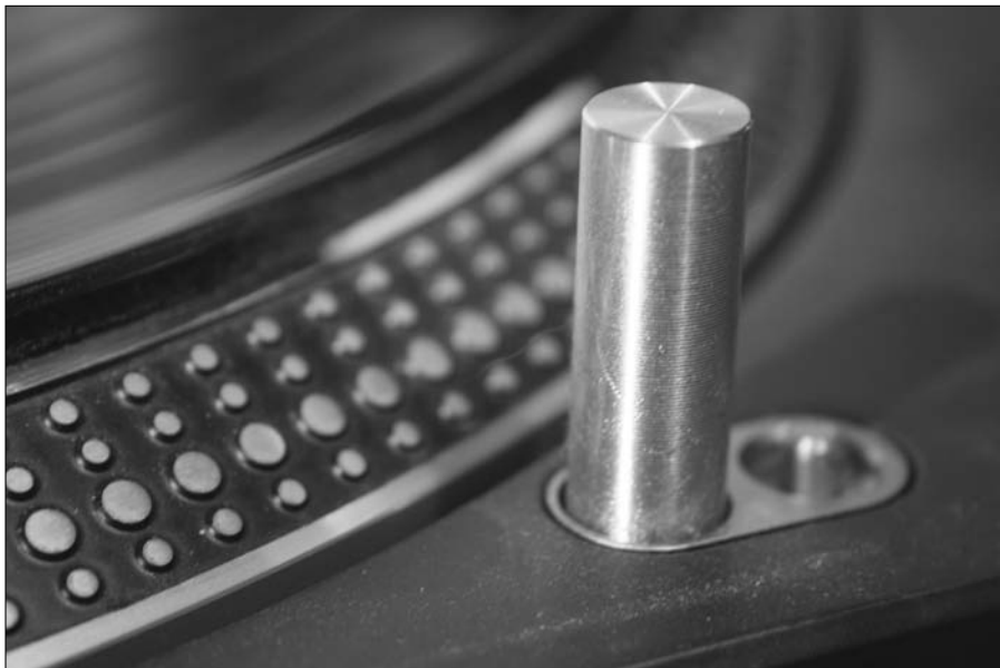
Figure 5-3: The target light on a Technics 1210. A helpful little fella.
