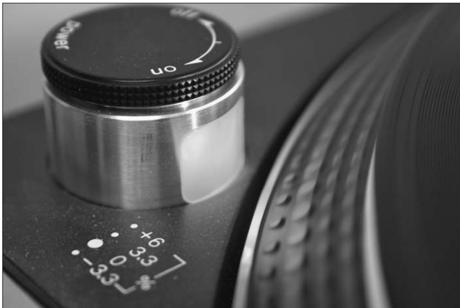
Figure 5-2: The strobe light on a Technics 1210.
