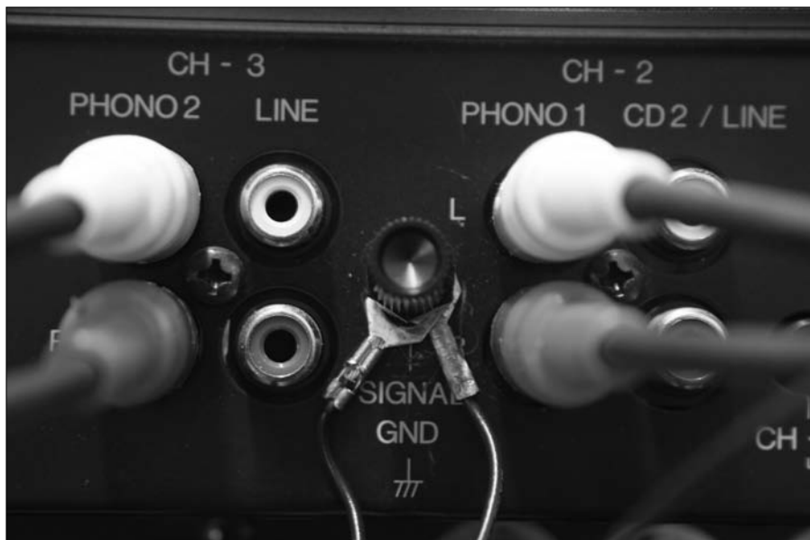
Figure 11-5: Two ground wires screwed to the back of the mixer.
