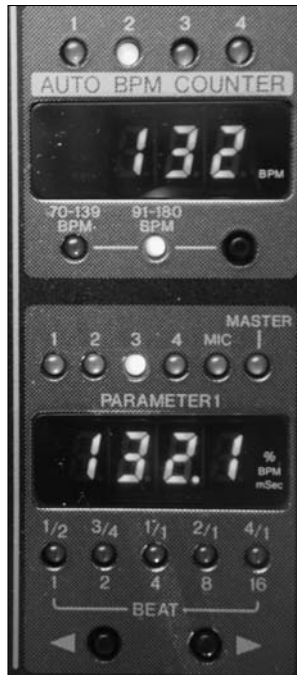
Figure 8-6: A built-in beat counter on the Pioneer DJM600.
