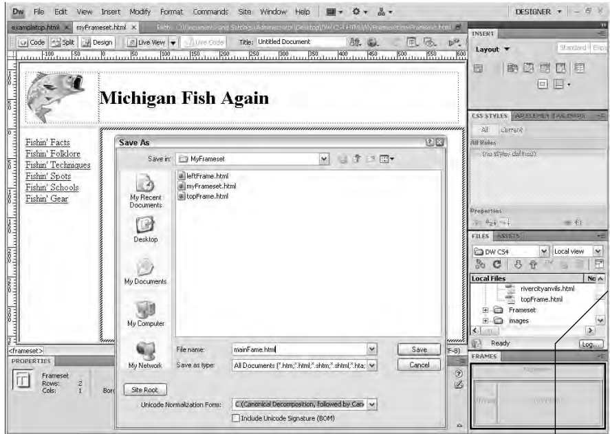
Figure 3-11: In Design view, a dark border appears around the frame being saved when you're saving the frameset and its files.
