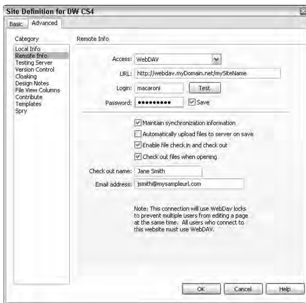
Figure 3-4: Enter the connected server's URL including protocol, port, and directory for WebDAV access.
