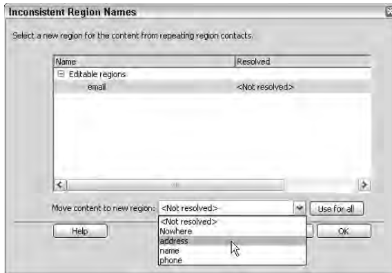
Figure 2-8: Use the Inconsistent Regions Names dialog box to map old editable region names to new editable regions.
