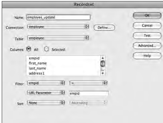
Figure 4-4: The Recordset dialog box configured to select only the record to update based on the specified URL parameter.
