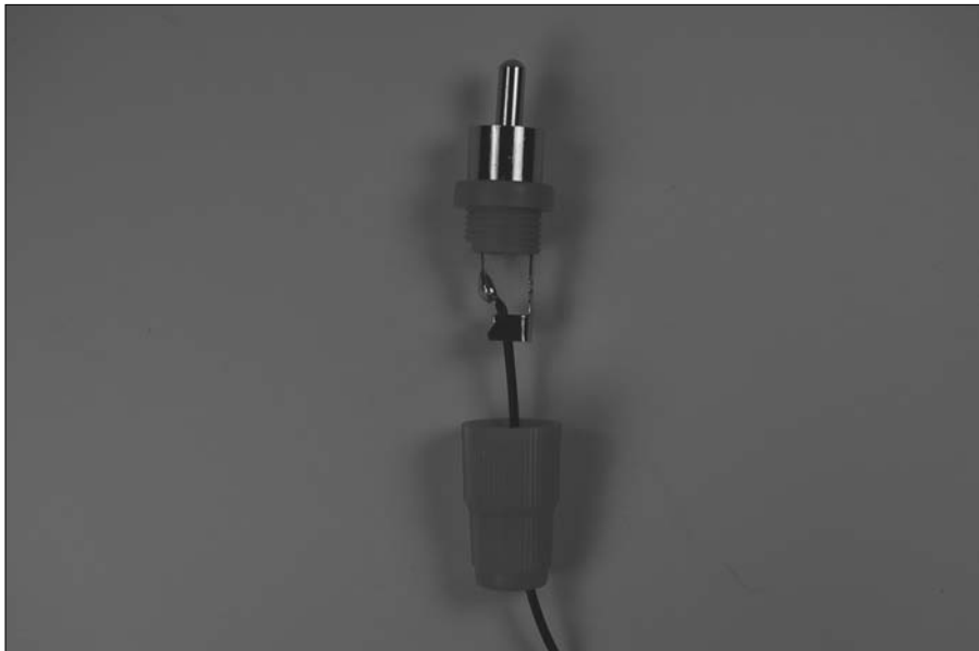
Figure 7-17: Solder wires to phono plugs.
