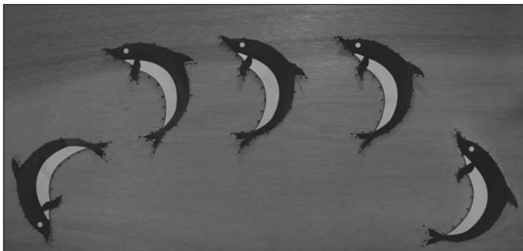
Figure 10-14: The plywood after drilling holes.
