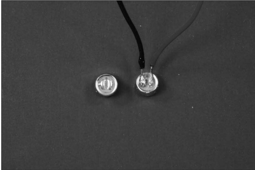
Figure 4-14: Soldering to flat contact pads.
