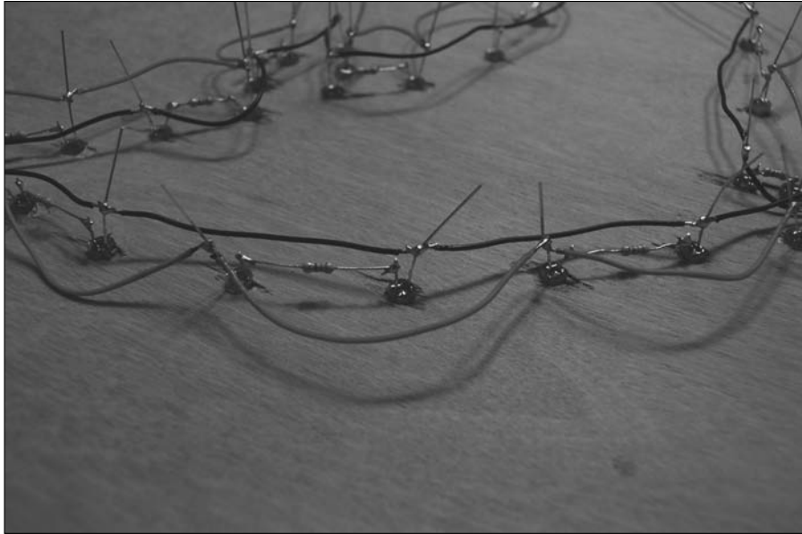
Figure 10-21: A close-up of red wires connecting long leads of LEDs.
