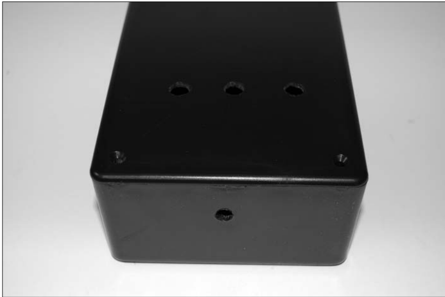
Figure 11-14: Drill holes for the LED and switches.
