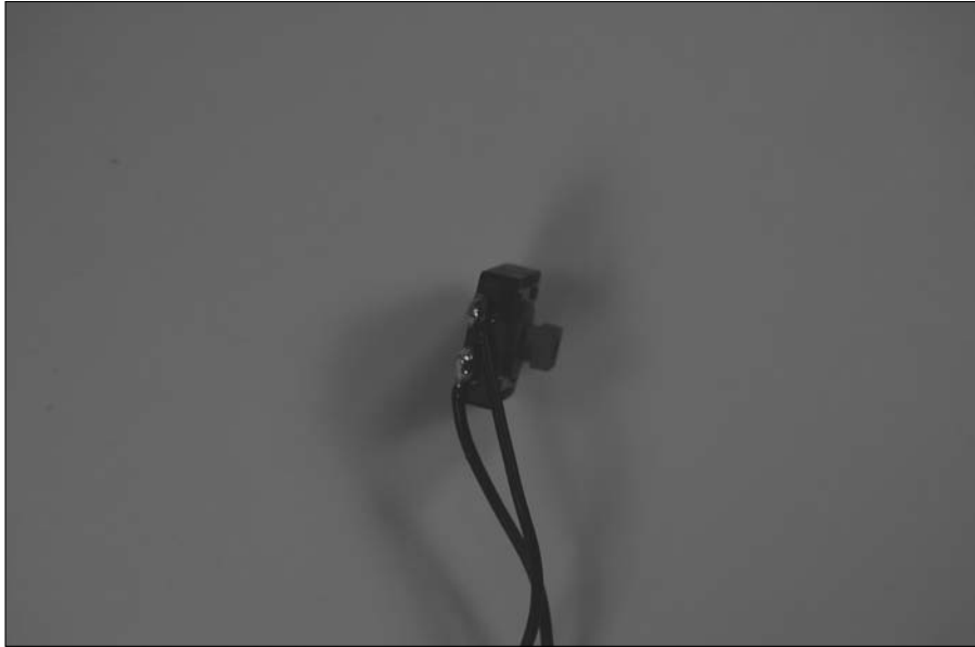
Figure 7-16: Solder wires to tactile switches.
