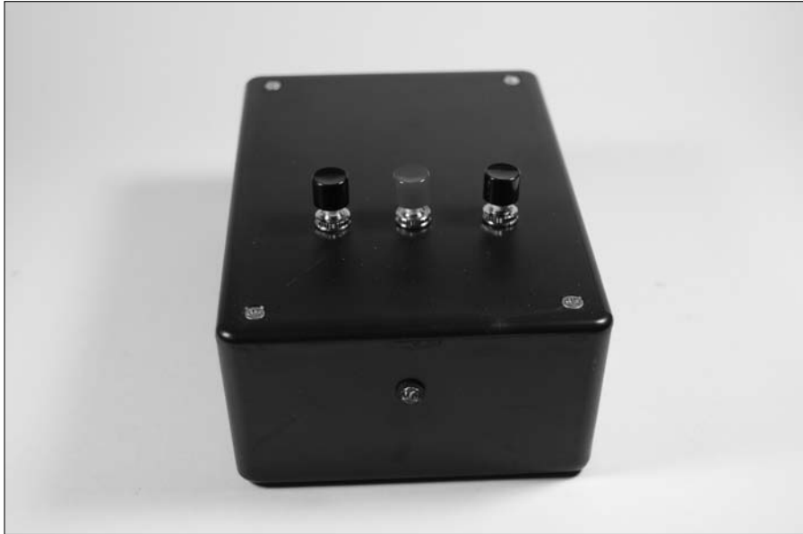
Figure 11-22: The transmitter all put together.
