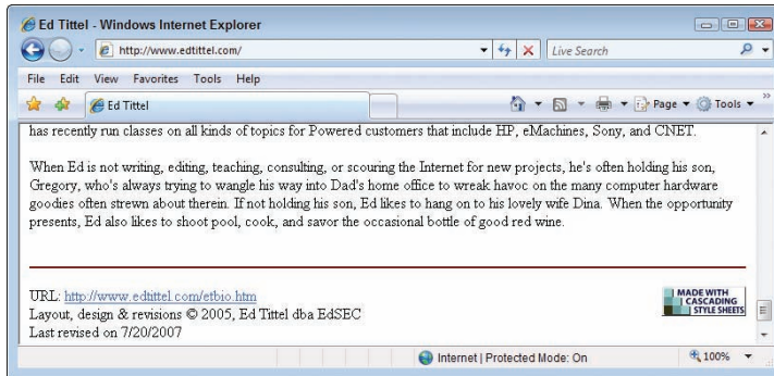
Figure 5-10: The EdTittel.com home page uses a colored rule to separate page content from page-footer information.
