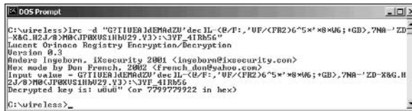
Figure 7-10: Cracking a WEP key stored in the Windows registry with the Lucent ORiNOCO Registry Encryption/ Decryption program.
