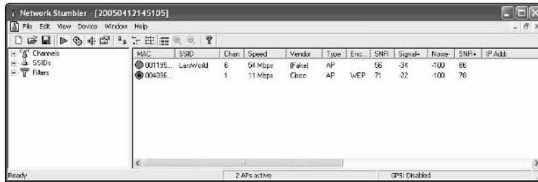
Figure 11-11: A Cisco AP with a hidden SSID in NetStumbler.
