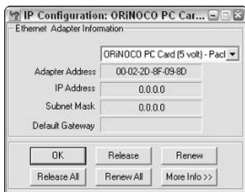
Figure 17-1: Using wntipcfg to release IP addresses.
