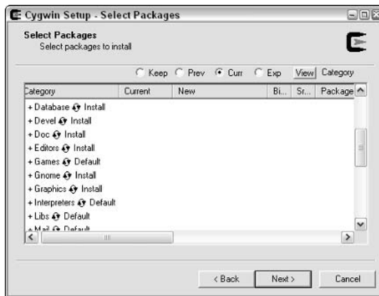
Figure 4-4: Selecting the packages to install.
