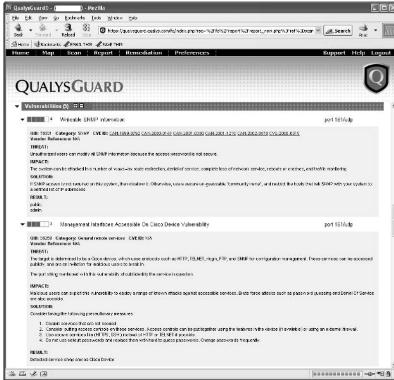
Figure 12-15: Qualys- Guard discovered that SNMP information is writable.
