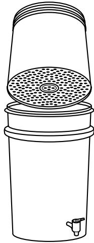
Figure 26-1: Assembling your own lauter tun.
