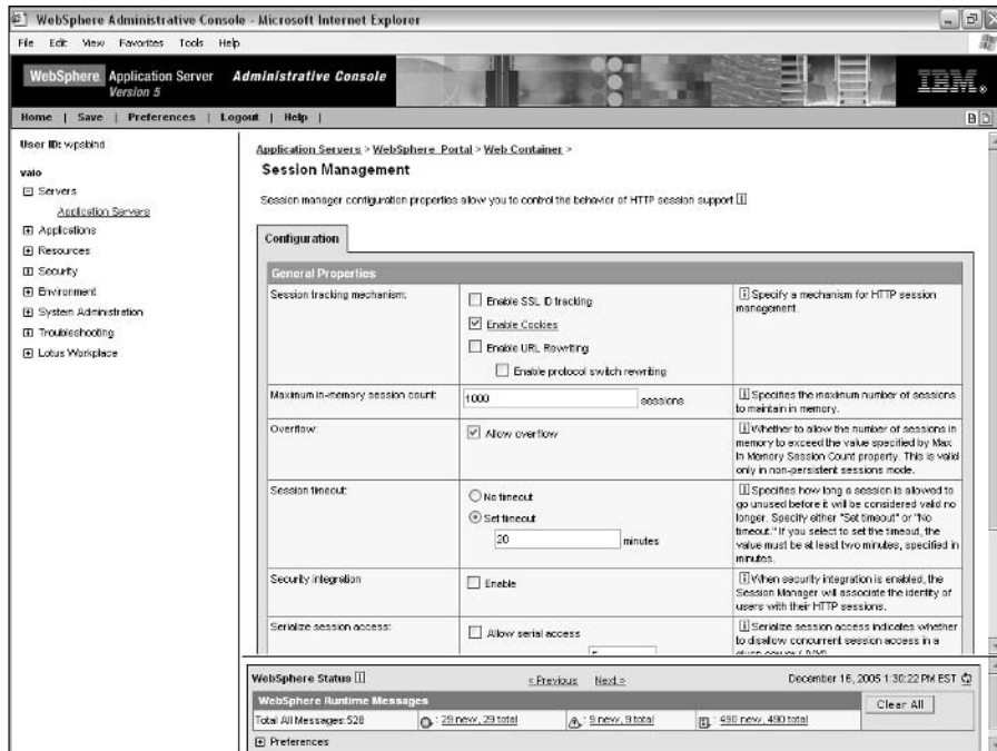
Figure 15-15: Use the WebSphere Adminis- trator to change the auto logout time period.
