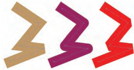
Figure 10-15: Three different joins on a path (left to right): Miter, Round, and Bevel.
