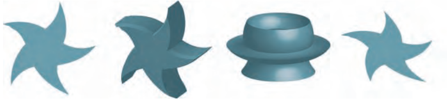
Figure 11-4: From left to right: Original path, extruded path, revolved path and rotated path.
