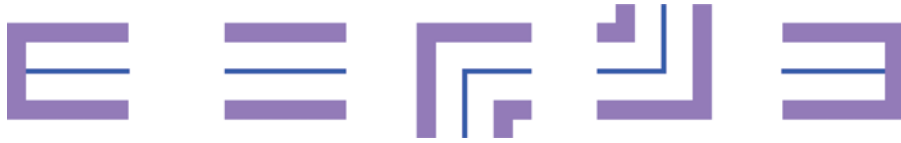
Figure 9-16: Left to right: Start, side, outside corner, inside corner, and end pieces.
