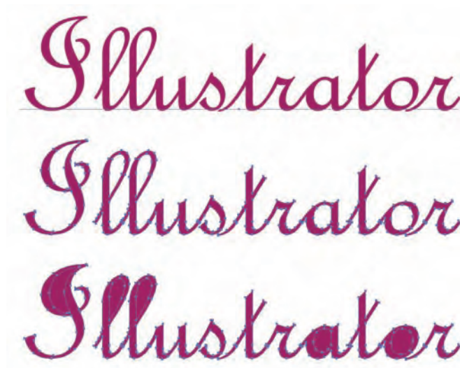
Figure 3-12: Text as text (top), as compound paths (middle), and as compound paths after release (bottom).
