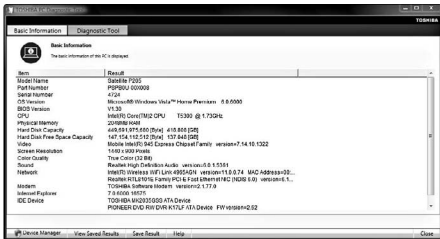
Figure 1-5: The Toshiba diagnostics information screen offers a quick inventory of the essential parts of your machine.
