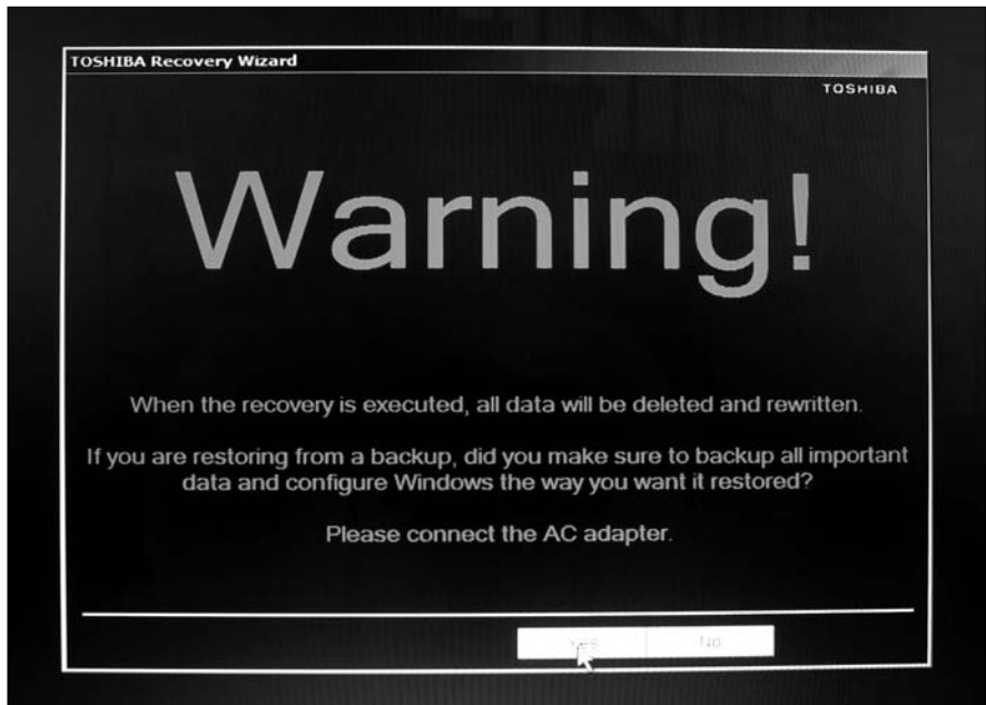
Figure 1-7: Reinstalling Windows from a recovery disc restores your machine to the way it came from the factory; that means all added programs, utilities, and files are wiped out. You've been warned!
