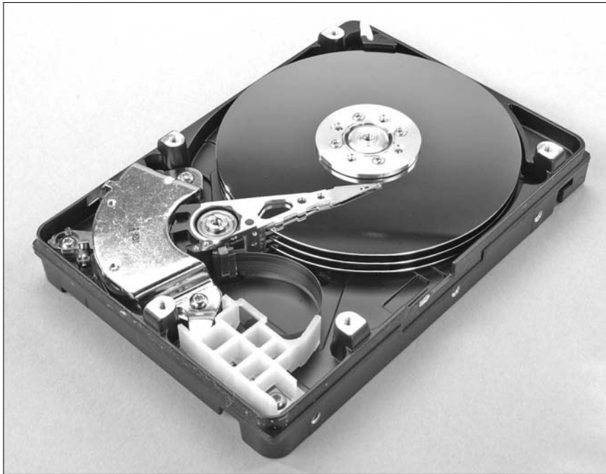
Figure 2-1: Its protective cover removed, here is the interior of a basic hard disk drive. This model, from a desktop computer, has three platters and six read-write heads that move in from the outside to the core.
