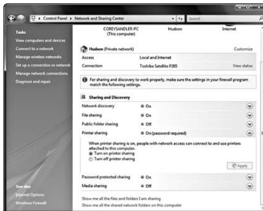
Figure 2-10: Windows Vista's Network and Sharing Center opens the door to printer sharing.
