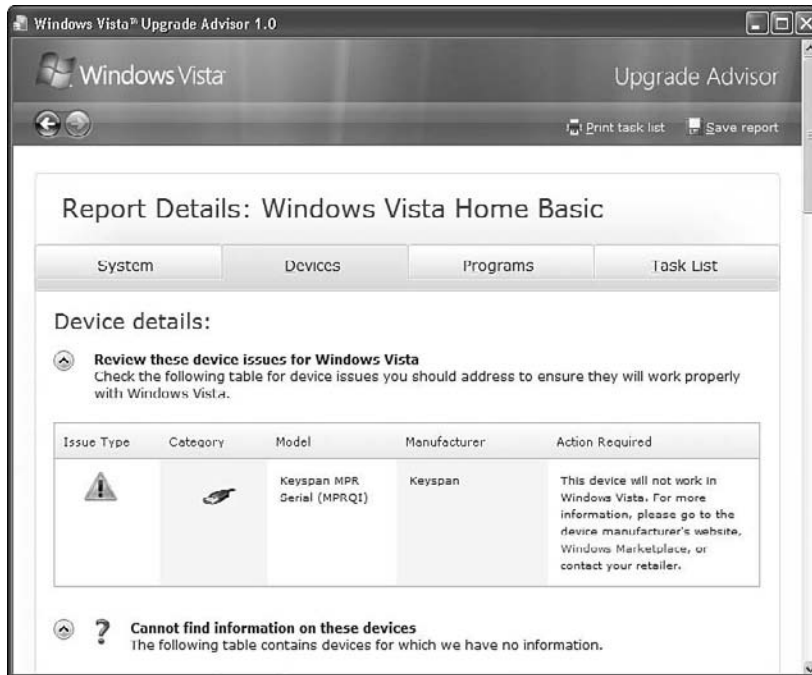
Figure 1-6: The detailed report of Windows Vista Upgrade Advisor shows that the operating system is incompatible with a particular piece of hardware.
