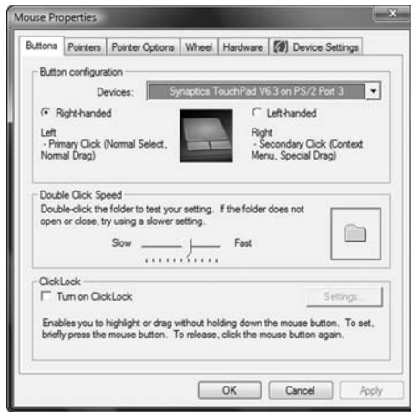
Figure 2-8: A Buttons tab for a Synaptics Touchpad in a Toshiba Satellite laptop.
