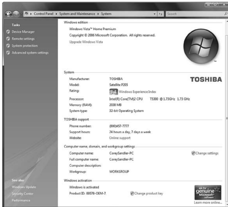
Figure 3-3: Toshiba's information screen includes the system's Windows Experience Index, its processor specs, memory, network configuration, and phone or online access to support technicians.
