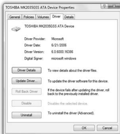
Figure 3-6: The Driver tab of Device Properties allows you to inspect, disable, uninstall, update, or roll back a device driver.
