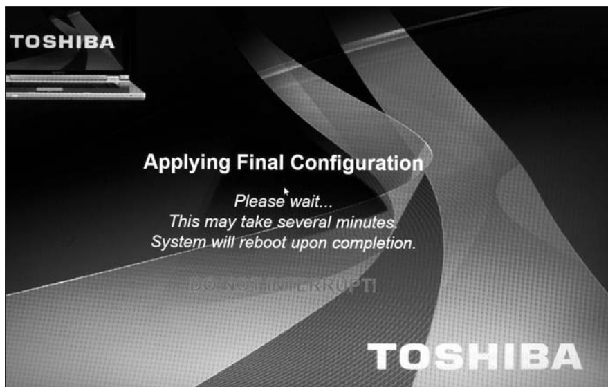
Figure 1-8: Are you paying attention? Never interrupt the process of recovering an operating system or installing a new one.
