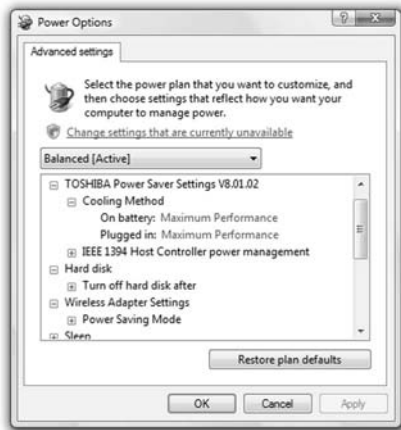
Figure 3-3: On the Toshiba Satellite P205 sample machine, the manufacturer has included advanced power saver settings for many individual components.
