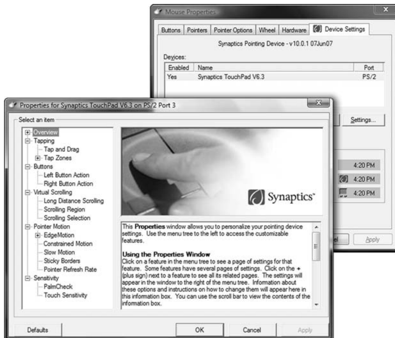
Figure 2-10: Advanced pointing device controls include adjustments to sensitivity of the touchpad and the use of “tap zones” to issue commands.
