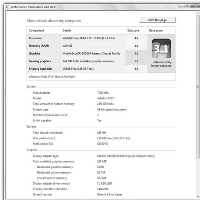
Figure 1-2: An examination of the subscores that lie beneath the base score for the Windows Experience helps pinpoint a machine's weakest link.
