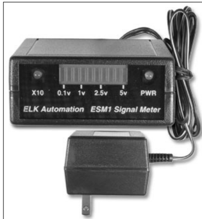
Figure 13-1: ELK ESM1- X10 Signal Meter.
