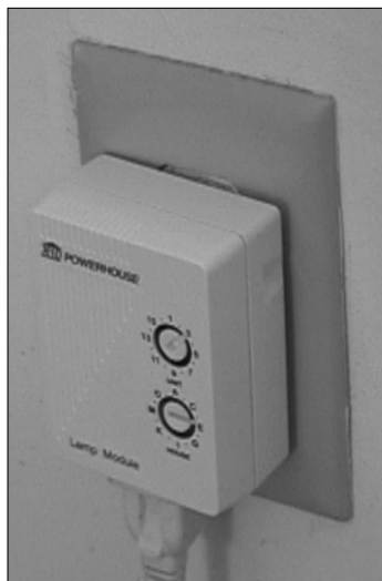
Figure 1-1: Use the X10 Lamp Module to control a light by using various X10 controllers.
