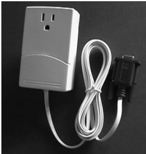
Figure 1-2: You can use the CM11A X10 computer interface with free Linux software to control your X10 modules.
