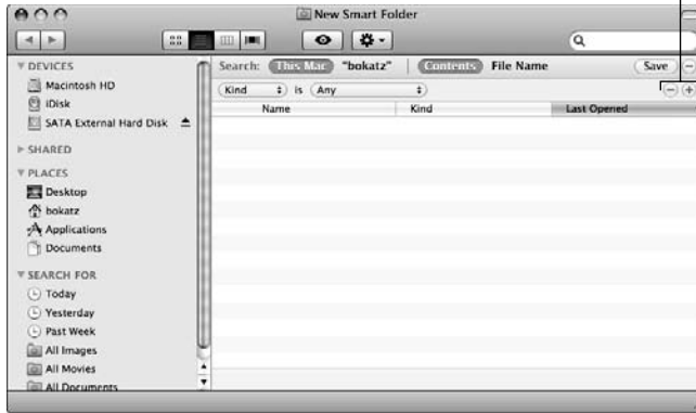
Figure 6-22: Clicking the plus sign icon displays a Kind and Any pop-up menu.
