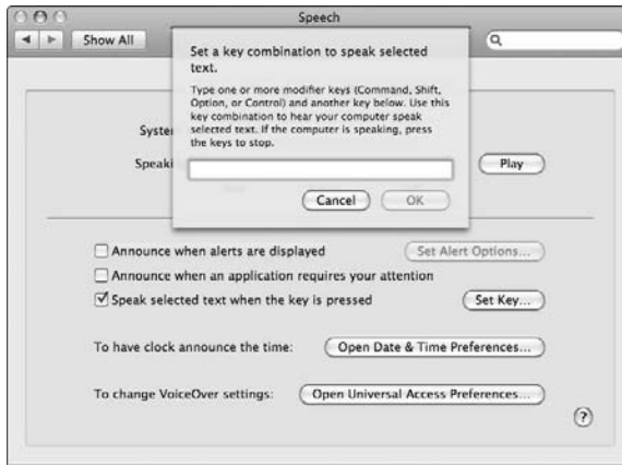
Figure 8-11: A dialog lets you define a keystroke combination to tell the Mac when to start speaking selected text.
