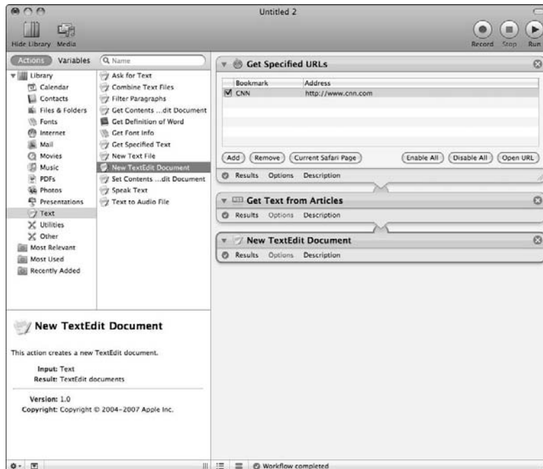
Figure 5-7: Three actions that retrieve RSS feeds from a Web page and display them in a TextEdit document.
