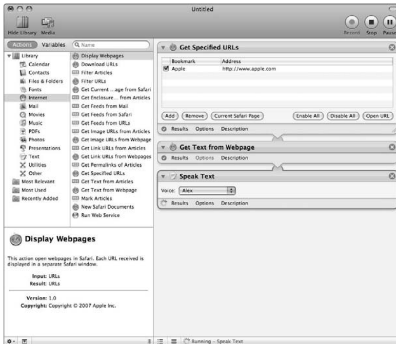
Figure 5-2: An action that processes data can output that data to an action that actually does something with that data.
