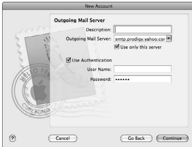
Figure 2-3: The Outgoing Mail Server dialog asks for the name of the server to send your e-mail through to the rest of the Internet.
