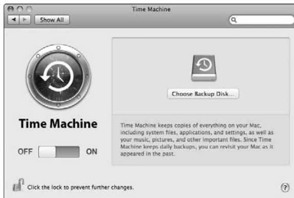
Figure 1-1: To set up Time Machine, you need to turn it on and choose an external drive to use.
