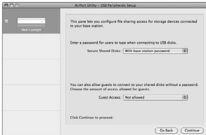
Figure 1-9: The dialog lets you set a password and access for an external hard drive.
