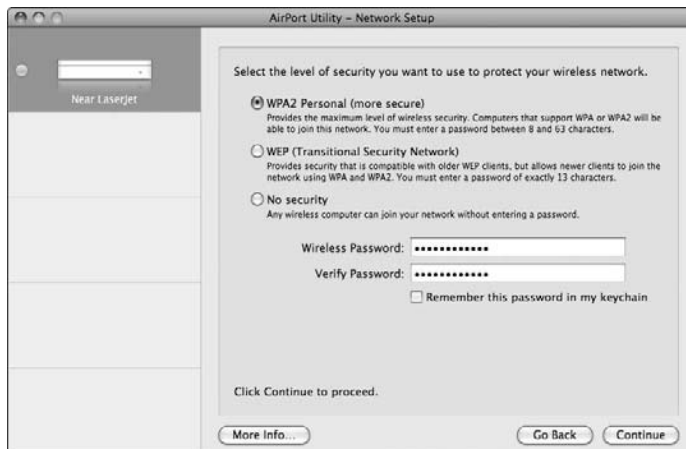
Figure 1-6: You can choose an encryption standard for scrambling your wireless network's signals.
