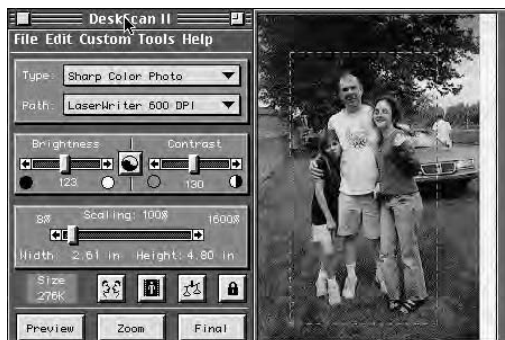
Figure 4-5: The software lets you crop a preview image to make it smaller and reduce the file size.
