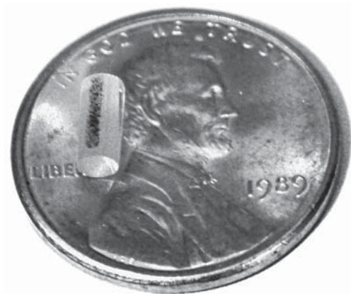
The Stanhope lens, shown against a penny, was one type of microdot reader issued by OTS.
