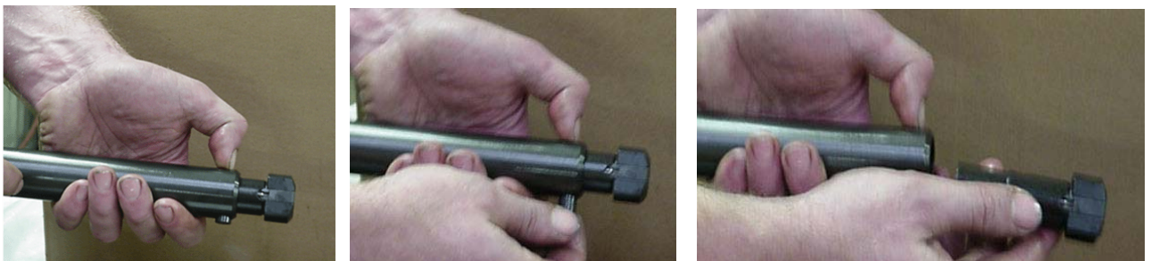
Figure 11, 12 & 13 Removing Bolt Retaining Pin to Remove Bolt Head
