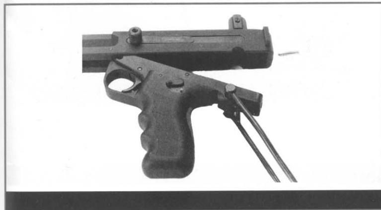
Lower sub-assembly separated from the receiver
