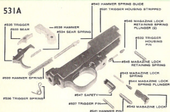
TRIGGER HOUSING ASSEMBLY
